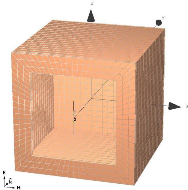
Figure 3. The method-of-moments model of the 200mm cell. The model does not include absorbing material at the back of the cell. Points 1 and 2 are the location of the two  $25 \Omega$  loads used to calculate the differential-mode and common-mode responses.
