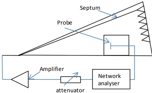
Figure 8. Measurement set-up in the GTEM cell.
