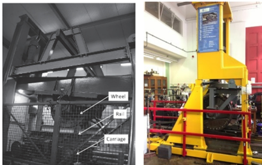
Figure 3- Full-scale test rigs at: left) voestalpine Schienen GmbH [19], right)
