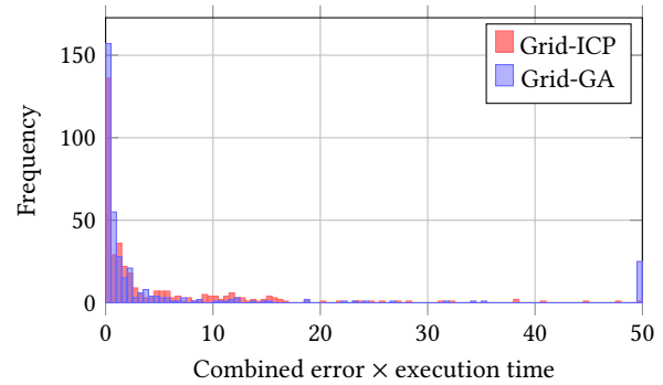
Figure 13: Histogram comparing the efficiency of Grid-ICP and Grid-GA algorithms
