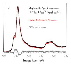
**Figure 3.** Fe  $L_{2,3}$ -edges of magnetite (a) and maghemite (b) samples (black). Also shown are linear reference fits (red) and difference spectra (grey) obtained by combining the previously measured iron valence and site standards (Figure 1) in the intensity ratios indicated by the formulae given in the figure legend and subtracting these from the experimental spectra.
