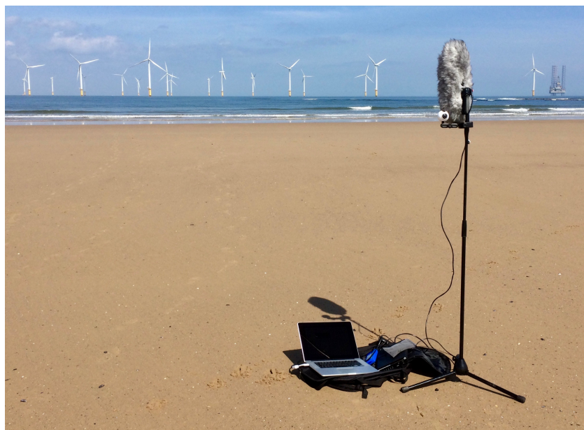
Figure 1. The setup used to record the EigenScape database: mh-Acoustics Eigenmike within Rycote windshield, Samsung Gear 360 camera, Eigenmike Microphone Interface Box and Apple MacBook Pro. The equipment is shown here at Redcar Beach, UK: 54°37'16" N, 1°04'50" W.
