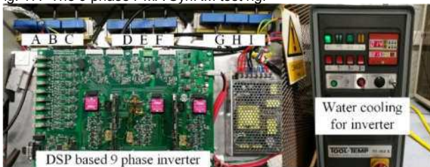
Fig. 18. DSP based 9 phase inverter.
