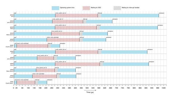
Fig. 3. Operating system and hardware latency measured for 40KiB and 80KiB reads from ext4, block device and CharlO storage
