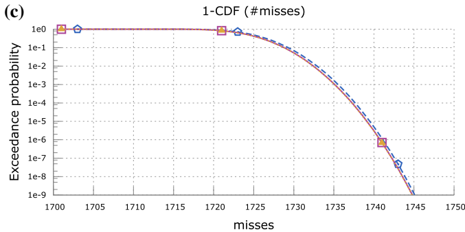
Estimated miss distribution for statemate, 275 distinct memory blocks, 1844 accesses on the longest path
