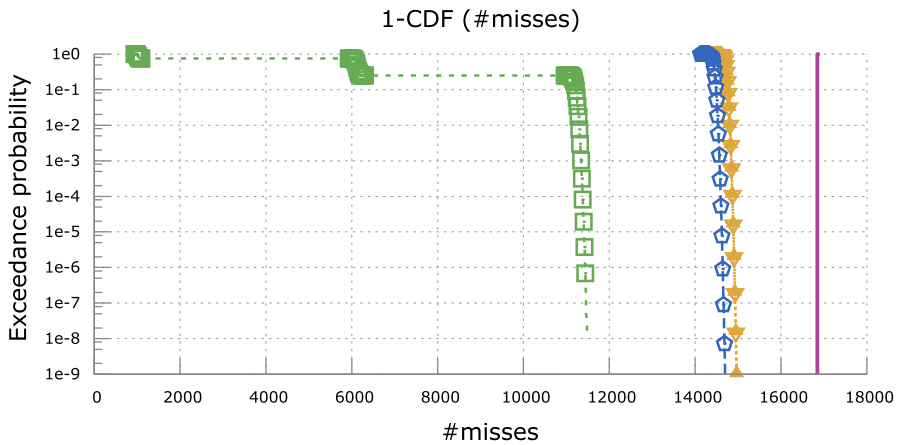
Fig. 18 Estimated miss distribution for fft under LRU and random replacement policies with analysed segments of M = 1000 potential misses (Color figure online)
