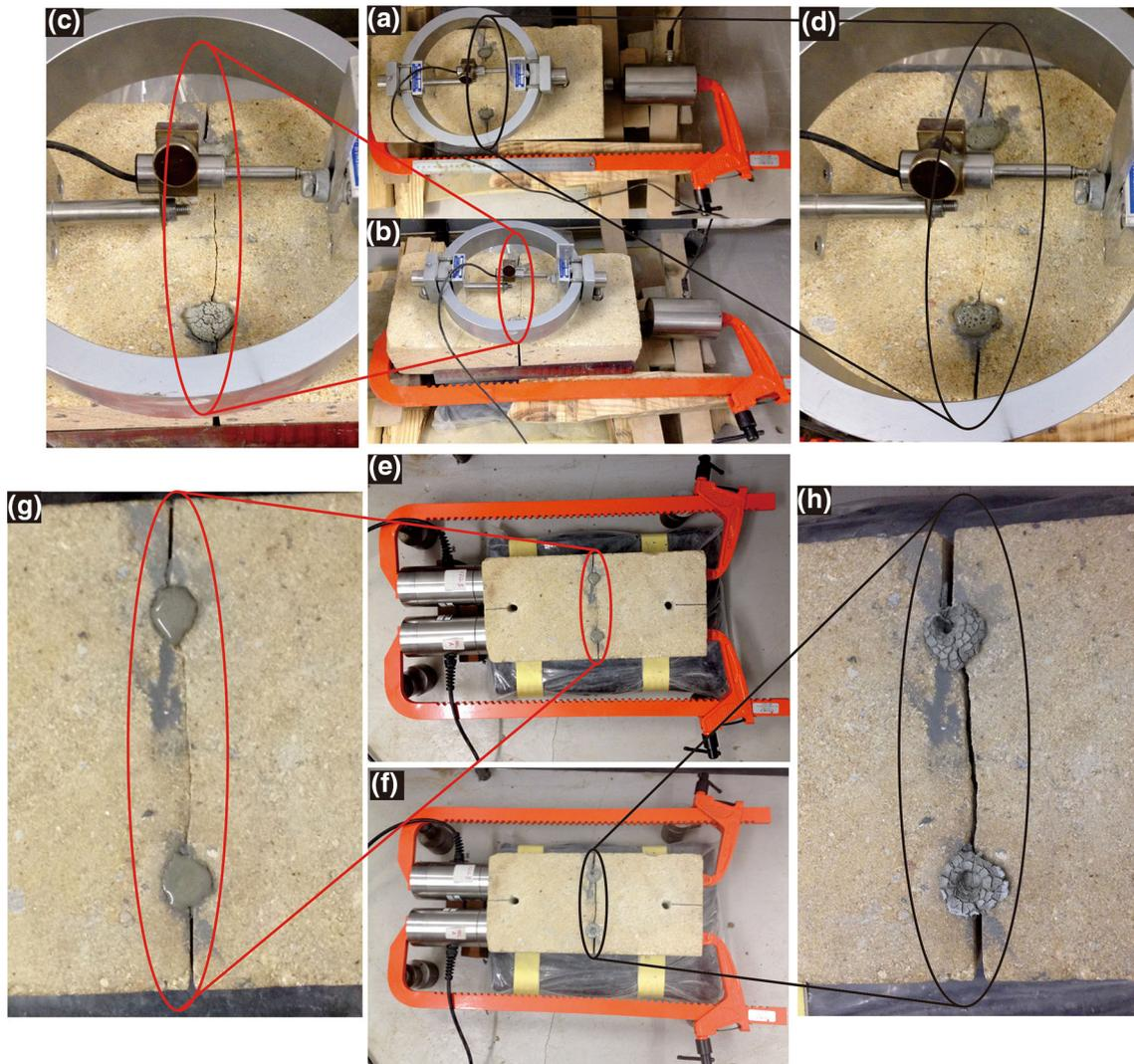
**Fig. 14** Phase ii tests conducted on the Midgley Grit Sandstone sample containing a mechanical fracture (**d** and **g**). The initiation (**a**) and completion (**b**) of the Type 1 re-setup tests. The initiation (**e**) and completion (**f**) of the Type 2 re-setup tests. The original induced fracture was re-opened (**c**) and (**h**)
