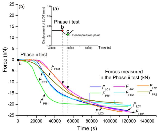
**Fig. 11** **a** Displacement of LVDT versus time measured in the Phase i test on the intact Thornhill Rock Sandstone sample and **b** measured force against time in the Phase ii test using the Type 1 re-setup method, in which forces were measured three times
