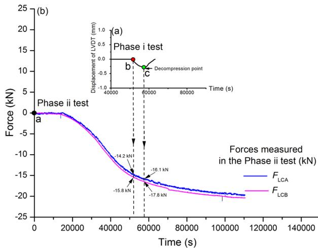
**Fig. 12** **a** Displacement of LVDT versus time measured in the Phase i test on the intact Thornhill Rock Sandstone sample and **b** measured force versus time in the Phase ii test using the Type 2 re-setup method
