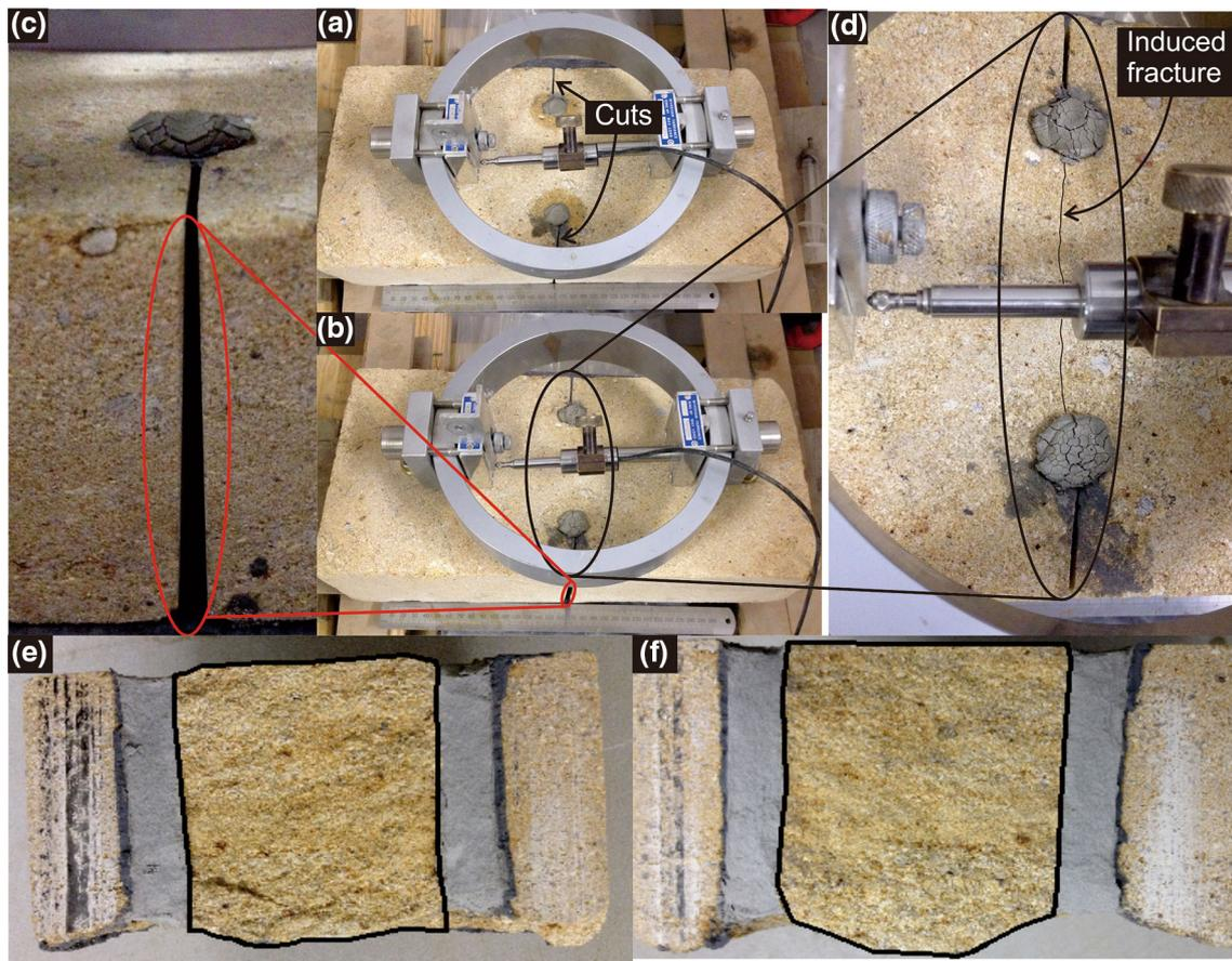
**Fig. 13** **a** Experimental setup of the Phase I tension test on an ostensibly homogeneous Midgley Grit Sandstone with additional twin cuts. **b** The completion of test, a cut on one side of the sample **(c)** and an induced fracture on the top surface **(d)**. Two opened failure surfaces are shown in **(e)** and **(f)**. Note that black-enclosed areas are used for tensile strength calculation
