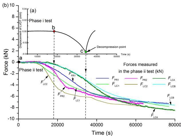
**Fig. 19** **a** Displacement of LVDT against time during the Phase i test on the incipient joint 2 within the BHQ 5 and **b** force versus time in the Phase ii test using the same sample but containing the previous opened fracture
