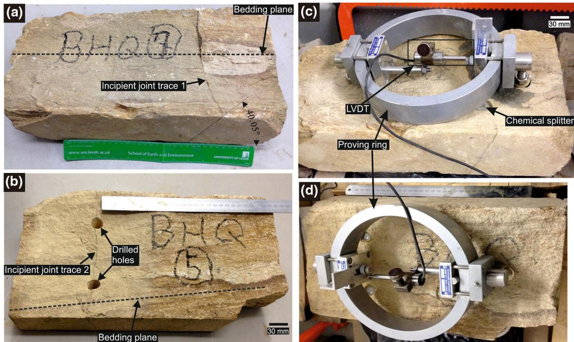
**Fig. 16** **a, b** Midgley Grit Sandstone samples (BHQ 7 and BHQ 5) containing the incipient joint traces 1 and 2. **c, d** Experimental setup of the tension tests on the samples with incipient joints
