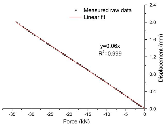
**Fig. 3** Relationship between force and displacement of the proving ring calibrated in Fig. 2
