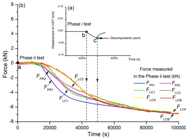
**Fig. 18** **a** Displacement of LVDT versus time during the Phase i test on the incipient joint 1 within the BHQ 7 and **b** force versus time in the Phase ii tests using the same sample but containing the previous opened fracture
