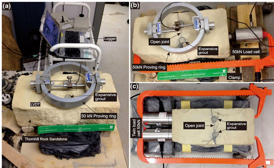
**Fig. 9** a Experimental setup of the Phase i test on an ostensibly homogeneous Thornhill Rock Sandstone sample and setups of the Phase ii test on the same sample but containing the opened fractures in the Phase i test using the Type 1 re-setup method (b) and the Type 2 re-setup method (c). Rule for scale is 350 mm in length
