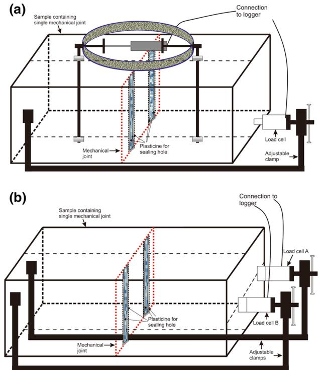
**Fig. 8** Diagram of the test setups on intact rock blocks containing fractures opened in the Phase i test (to measure ETF). a The Type 1 re-setup method and b the Type 2 re-setup method. Figure not to scale
