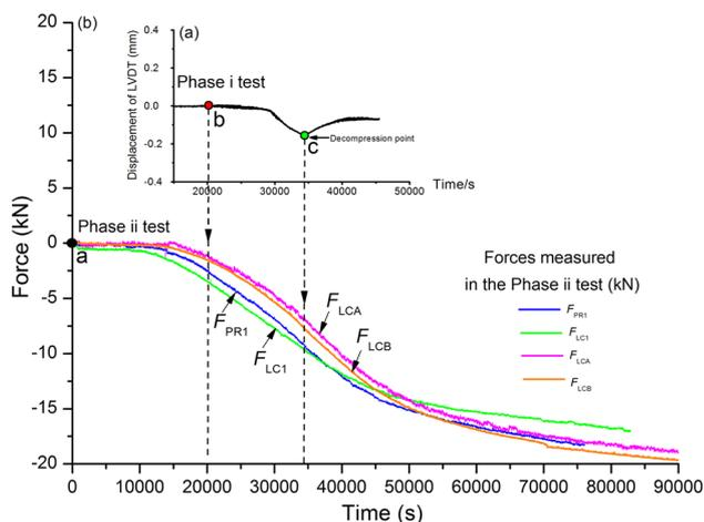
**Fig. 15** **a** Displacement of LVDT versus time during the Phase i test on the Midgley Grit Sandstone sample and **b** force against time in the Phase ii test using the same sample but containing the previous opened fracture
