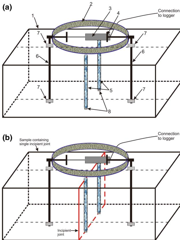
**Fig. 7** Diagram of the test setups on intact rock blocks without (a) and with an incipient joint (b). 1—Intact rock sample without incipient joint; 2—a proving ring (50 kN); 3—LVDT; 4—LVDT holder; 5—chemical splitter; 6—threaded rods; 7—nuts; 8—spectrum plasticine on the bottom. Figure not to scale
