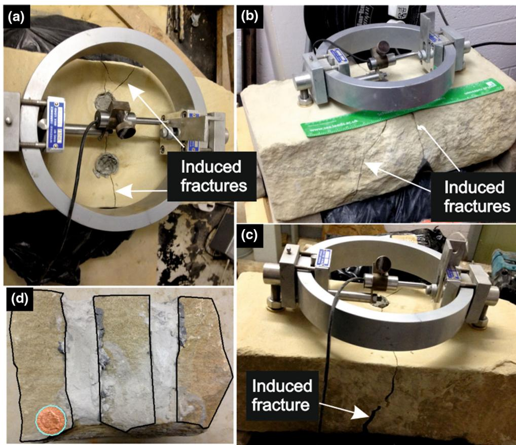
**Fig. 10** Failure patterns of the Thornhill Rock Sandstone sample under tension in the Phase i test described in Fig. 9a. **a** Front view; **b** left view; **c** right view; and **d** one failure plane (enveloped areas) used for the tensile strength calculation
