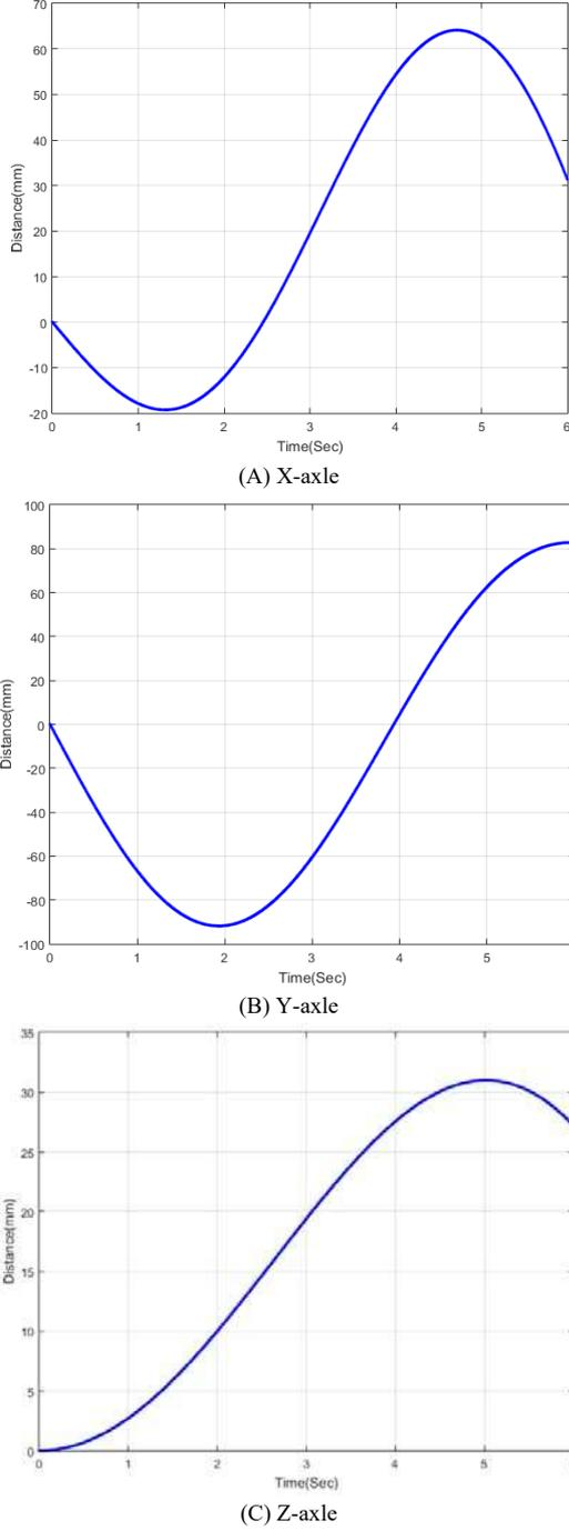
Figure 2. Trajectory of tool mounting bracket (Joint 7)
