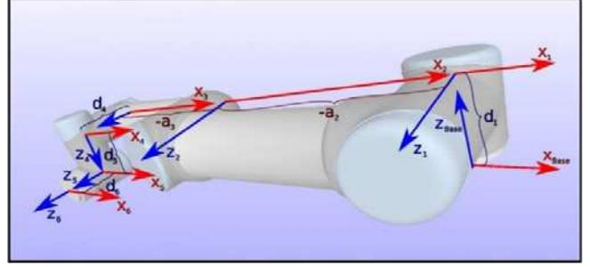
Figure 1. The Definition for centre of mass parameters [1]
