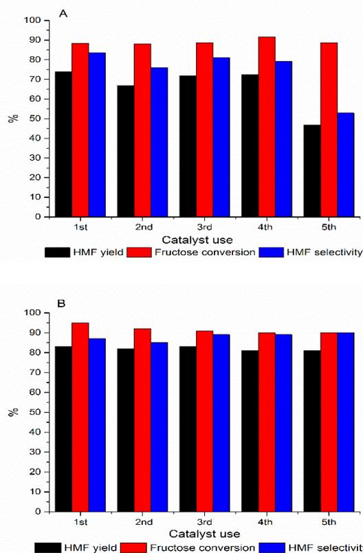
Figure 15. Reusability data for Fructose conversions, HMF yields and selectivities over Fe-NHC expanded HACS (**1a**, Top A) and Fe-NHC Starbon 350 (**1b**, Bottom B). Conditions: D-fructose (180 mg, 1mmol), Fe-NHC (**1a**) (38 mg, 0.01 mmol) Fe-NHC (**1b**) (32 mg, 0.01 mmol) at 100 °C in DMSO- $d_6$  (4 mL), time 1 h.
