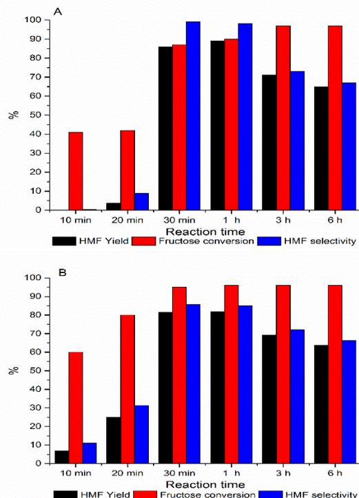
Figure 14. Fructose conversion, HMF yields and selectivity over Fe-NHC expanded HACS (**1a**, Top A) and Fe-NHC Starbon 350 (**1b**, Bottom B) catalysts. Conditions: D-fructose (180 mg, 1mmol), Fe-NHC (**1**) (32 mg, 0.01 mmol) at 100 °C in DMSO- $d_6$  (4 mL).
