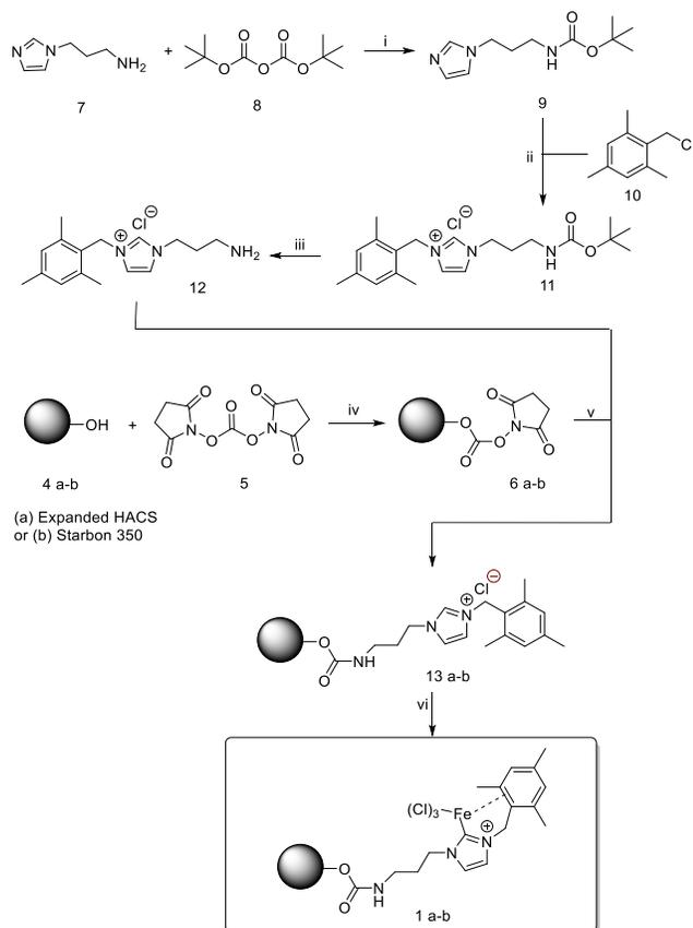
Figure 1. Synthetic route to iron-NHC catalysts 1a and 1b.
