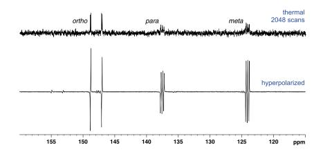
**FIGURE 3** *Top*: Thermal  $^{13}$ C NMR spectrum of **3a** (100 mM) and SABRE catalyst (5 mM) in methanol- $d_4$  after 2,048 scans. Bottom: single-scan hyperpolarized  $^{13}$ C NMR spectrum
