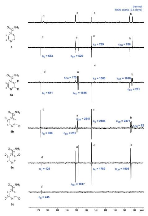
**FIGURE 6** Series of hyperpolarized single-scan  $^{13}$ C NMR spectra of **5–5d** (100 mM) and [IrCl(COD)(IMes)] (5 mM) in methanol- $d_4$  under p-H<sub>2</sub> after transfer at 0.5 G. Thermally polarized reference  $^{13}$ C NMR spectrum (top), acquired over 4,096 scans.  $\varepsilon$  = enhancement factor, fold gain
