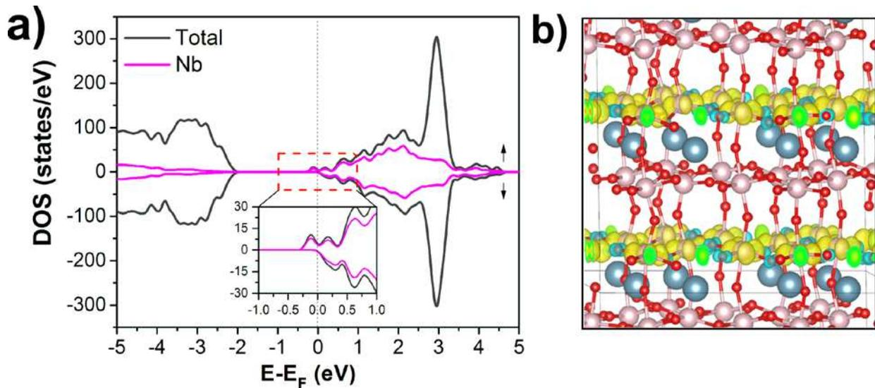
**Figure 11:** a) DOS and b) spin density iso surface of  $1.4 \cdot 10^{-3} \mu_B/\text{\AA}^3$  for oxygen deficient  $\text{La}_{1/3}\text{NbO}_{3-\delta}$  ( $\delta=0.02$ ). An approximate position of the oxygen vacant site is shown by a dashed circle.
