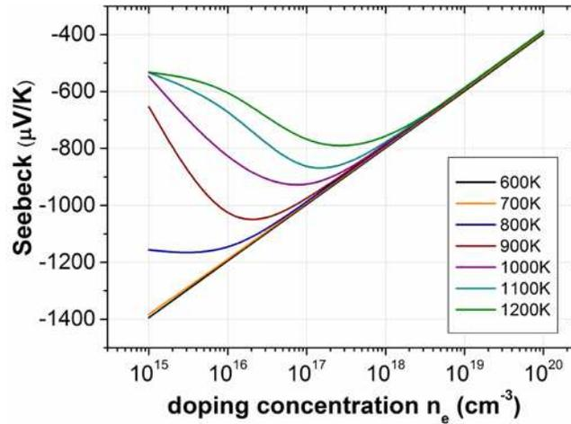
**Figure 10:** Calculated Seebeck coefficient dependence on the doping concentration for various temperatures, using a rigid-band model that assumes no shape change in the band structure, but only a shift in the Fermi energy due to the changing electron doping concentration.
