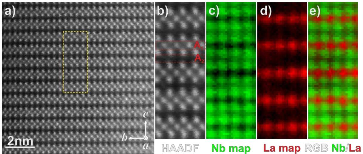
**Figure 4:** Example of atomically-resolved EELS measurement of the LNO ceramic, performed along the  $[100]$  zone axis: a) HAADF STEM Survey image, showing the area used for analysis marked by a yellow rectangle, b) HAADF STEM signal intensity acquired simultaneously with the EELS signal, c) integrated EELS intensity map of the Nb  $L_{2,3}$  edge, d) integrated EELS intensity map of the La  $M_{4,5}$  edge and e) RGB overlay of the Nb and La maps.
