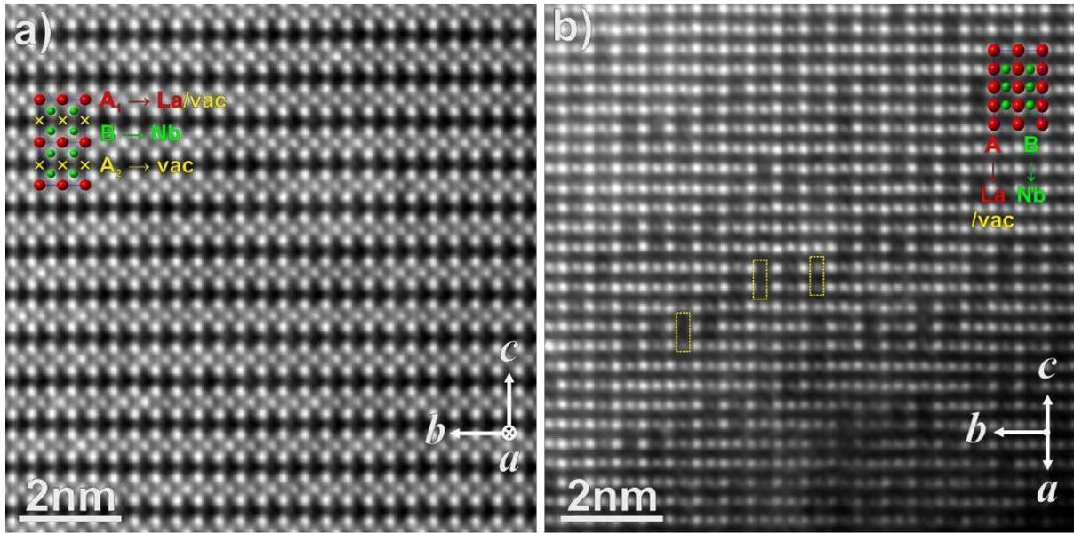
**Figure 3:** HAADF STEM images (averaged by non-rigid registration<sup>23</sup> from a stack of 50 consecutive frames) of the LNO ceramic acquired along the a) [100] and b) [101] zone axes. The corresponding ball-and-stick models of the LNO  $Cmmm$  structure<sup>29</sup> (oxygen positions not shown), are overlaid on the images for comparison (where yellow  $\times$  symbols denote the vacant  $A_2$  sites).
