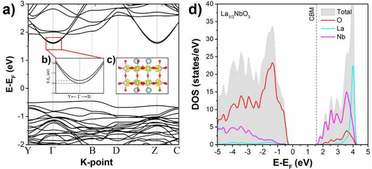
**Figure 7:** a) PBE+ $U$  band structure along the symmetry directions of the Brillouin zone. The high symmetry k-points of the primitive cell are:  $Y$  ( $1/2, 0, 0$ ),  $\Gamma$  ( $0, 0, 0$ ),  $B$  ( $0, 0, 1/2$ ),  $D$  ( $0, 1/2, 1/2$ ),  $Z$  ( $0, 1/2, 0$ ) and  $C$  ( $1/2, 1/2, 0$ ). b) Conduction bands in the vicinity of  $\Gamma$ . c) Charge density plot of the lowest conduction band. d) Total density and projected density of states of LNO. The CBM is indicated by the dashed lines.
