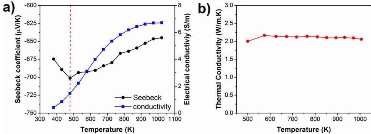
**Figure 6:** Experimental thermoelectric properties of LNO as a function of temperature. a) Measured Seebeck coefficient and electrical conductivity; the red line indicates the temperature for which the Seebeck coefficient has the highest value; b) Experimentally determined lattice thermal conductivity.
