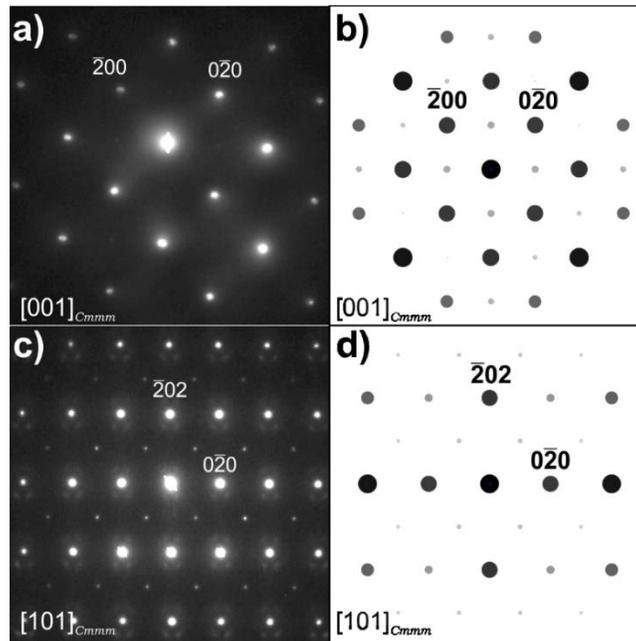
**Figure 2:** Experimental SAED patterns acquired along the (a)  $[001]_{Cmmm}$  and c)  $[101]_{Cmmm}$  zone axes, and corresponding simulated patterns in panels (b) and (d), respectively. The experimental diffraction patterns only show the characteristic diffuse satellite reflections along the  $[22\bar{2}]$  direction.
