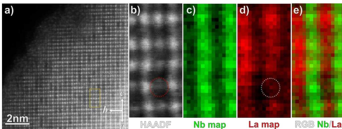
**Figure 5:** Example of atomically-resolved EELS measurement of the LNO ceramic, performed along the  $[101]$  zone axis: a) HAADF STEM Survey image, showing the area used for analysis marked by a yellow rectangle, b) integrated HAADF STEM signal intensity acquired simultaneously with the EELS signal, c) integrated EELS intensity map of the Nb  $L_{2,3}$  edge, d) integrated EELS intensity map of the La  $M_{4,5}$  edge and e) RGB overlay of the Nb and La maps.
