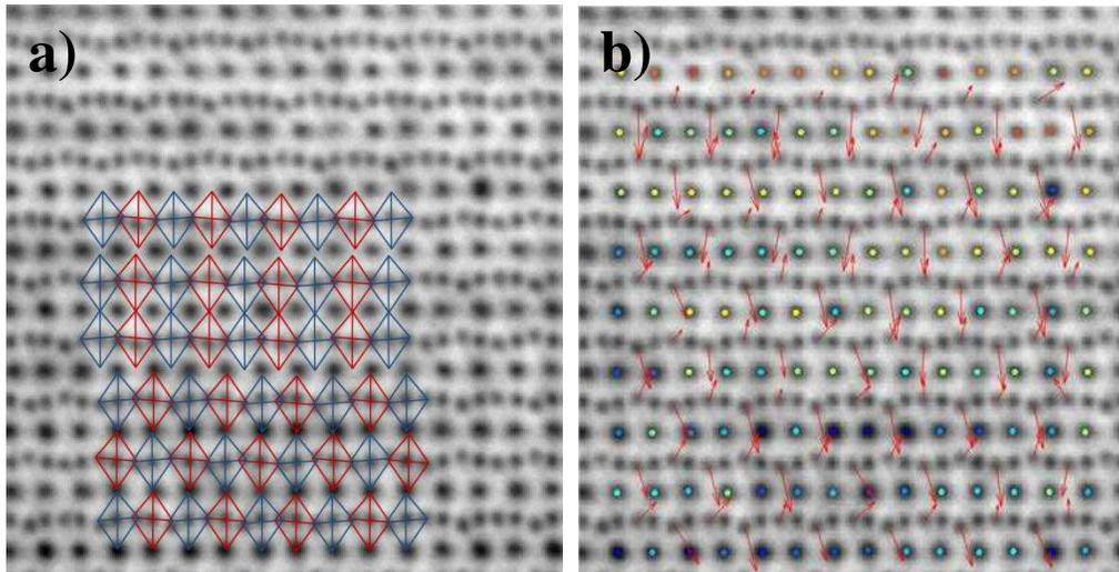
**Figure 1.** a) Annular Bright Field Image of a  $\text{Nd}_{2/3x}\text{TiO}_3$  ceramic acquired along the [110] zone axis, showing change in the  $\text{TiO}_6$  octahedral ordering and b) the same image showing relative displacements of the O sublattice positions.
