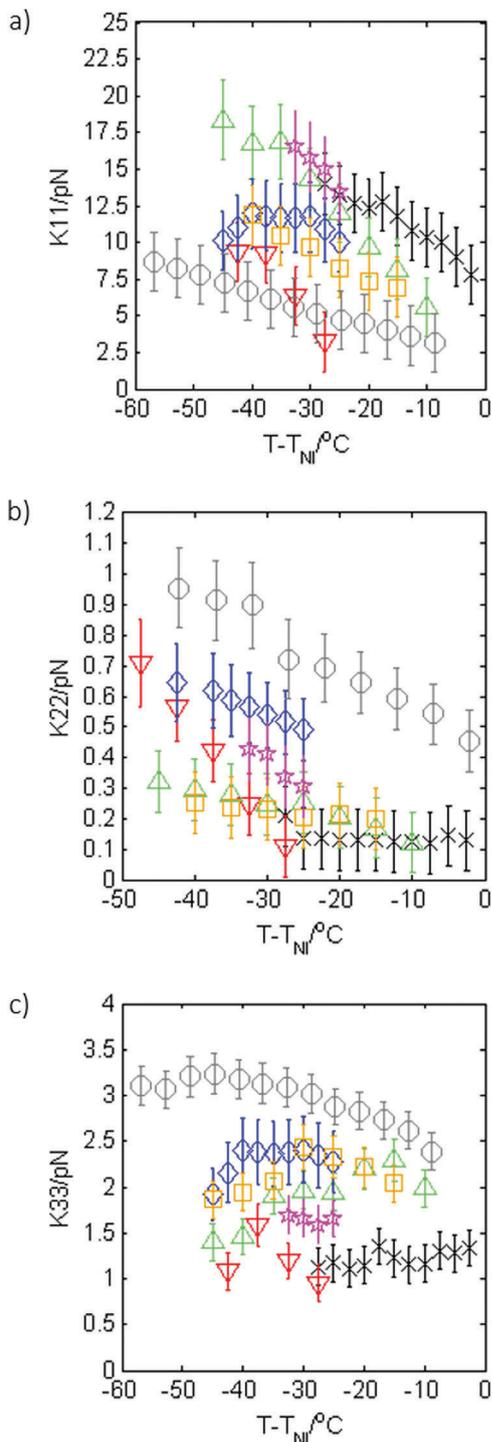
Fig. 9 The splay,  $K_{11}$  (a), twist,  $K_{22}$  (b) and bend,  $K_{33}$  (c) elastic constants as a function of  $T - T_{NI}$  for compound **1** (black crosses), compound **2** (grey circles), mixture 1 (red downward triangles), mixture 2 (green upward triangles), mixture 3 (blue diamonds), mixture 4 (orange squares) and mixture 5 (magenta stars).
