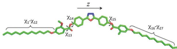
Fig. 3 Molecular structure of compound **1** without hydrogen atoms. Arrows show the dihedral ( $\chi_i$ ) allowed to rotate in the Monte Carlo conformation sampling. The molecular frame  $\{x, y, z\}$  has the  $z$  axis passing through the carbon atoms of the oxadiazole ring and  $y$  perpendicular to the plane of the ring.
