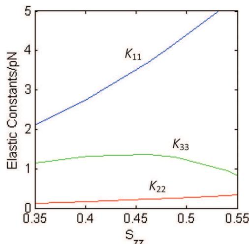
Fig. 7 Elastic constants calculated for the nematic phase of compound **1** as a function of the orientational order parameter  $S_{zz}$ , which quantifies the alignment of the  $z$  molecular axis (see Fig. 3) to the nematic director.
