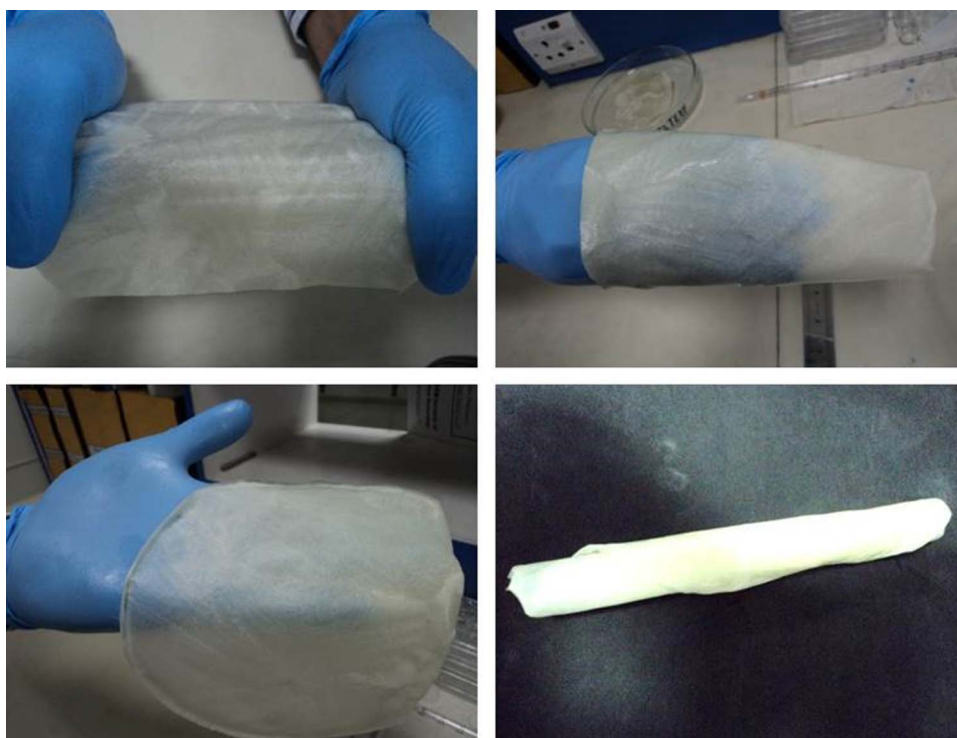
Fig. 1. Photographs of chitosan (CS)/collagen hydrogels to show their shape, flexibility, and ability to be folded.
