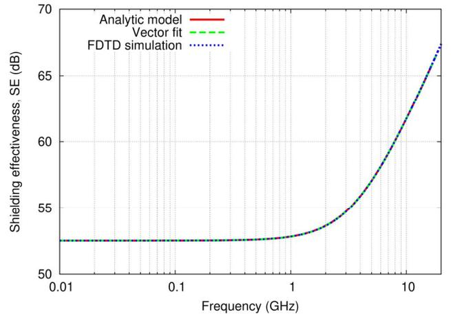
Fig. 6. Shielding effectiveness of an isotropic metalized fabric.
