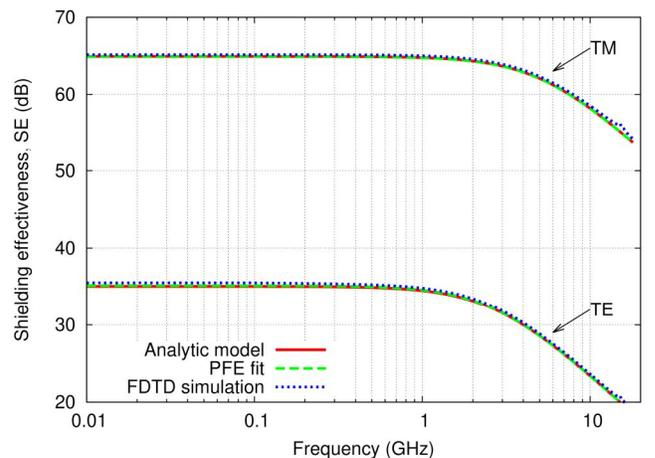
Fig. 7. Shielding effectiveness of an anisotropic wire mesh.
