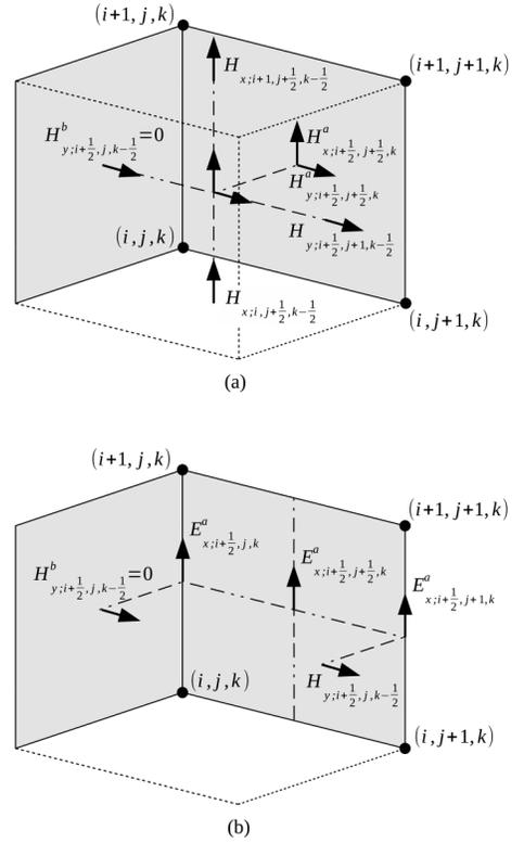
Fig. 5. Intersection between two SIBC faces (shaded) in the face centric approach showing the fields involved in: (a) The tangential magnetic field update adjacent to the SIBC; (b) The tangential electric field update on the SIBC.
