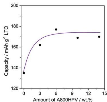
**Fig. 8.** Variation of specific capacity of LTO at 58 mA g<sup>-1</sup> as function of the amount of A800HPV added in electrode formulation.
