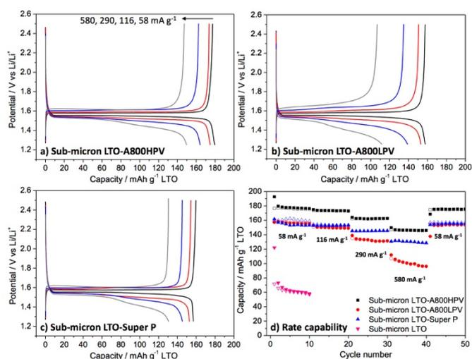
**Fig. 9.** Galvanostatic charge-discharge voltage profile (1.25 to 2.5 V) of a) Sub-micron LTO-A800HPV, b) Sub-micron LTO-A800LPV and c) Sub-micron LTO-Super P. d) Rate-capability and cycling performances at different current (58, 116, 290 and 580 mA g<sup>-1</sup>). Sub-micron LTO electrodes prepared without any carbon additive tested only until 10<sup>th</sup> cycle at 58 mA g<sup>-1</sup>. Filled and open symbols refer to reduction (discharge) and oxidation (charge), respectively.
