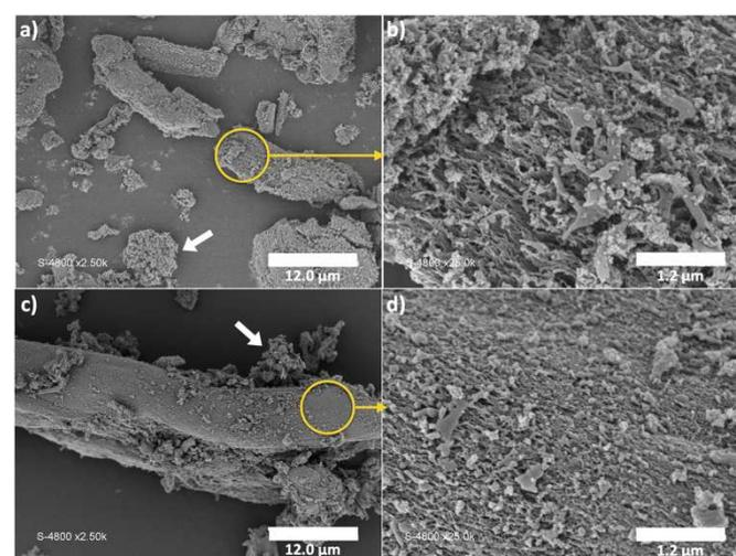
Fig. 1 SEM image of a) A800HPV, b) zoomed image of selected zone of A800HPV (fibre-like aggregates), c) A800LPV and d) zoomed image of selected zone of A800LPV (fibre-like aggregates); foam-like aggregates indicated by white arrow. For other carbon additives, such as A800MPV or Super P, see Fig. S6.
