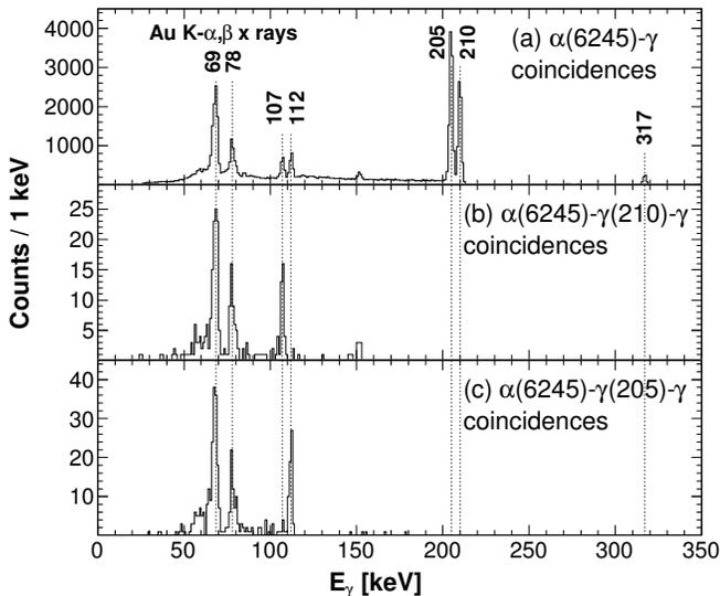
FIG. 5. Gamma rays in coincidence with: (a) the 6245-keV  $\alpha$ -decay transition, (b) the 6245-keV  $\alpha$  and 210-keV  $\gamma$  decay and (c) the 6245-keV  $\alpha$  and 205-keV  $\gamma$  decay. The energy range used as the  $\alpha$  gate was 6220–6320 keV.
