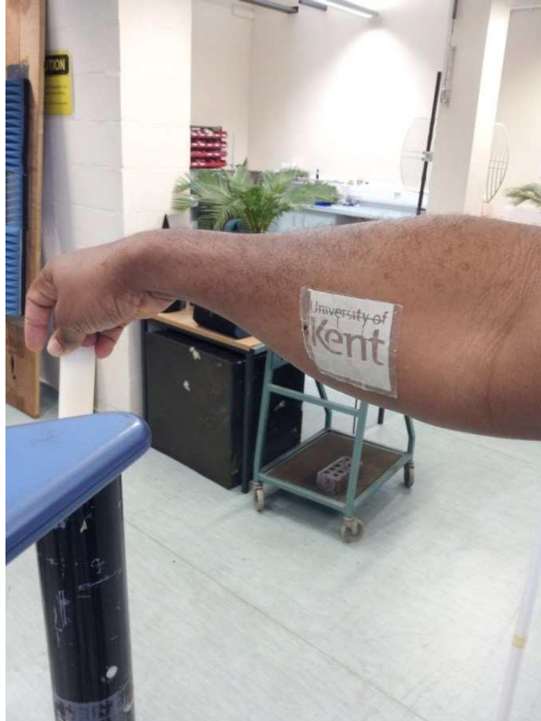
Fig. 8. Read range measurement of Kent logo tag
