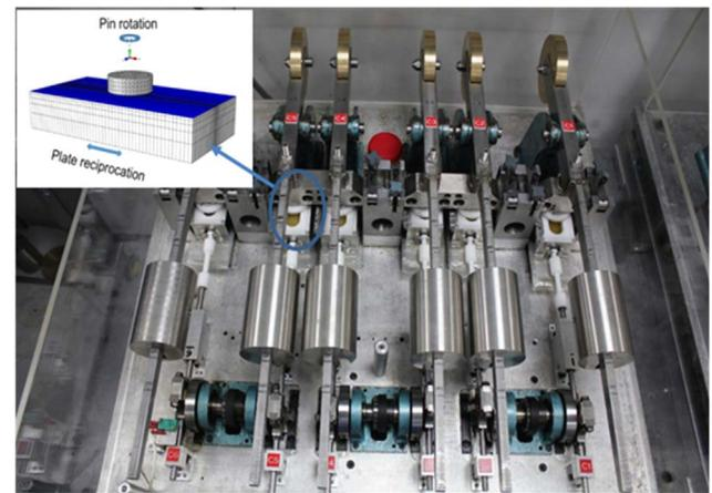
Fig. 2. Multidirectional pin-on-plate wear simulator.
