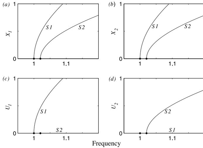
Fig. 4. Backbone curves for the two degree-of-freedom example showing the backbone curves in both physical space (a) & (b) and in the normal form coordinates (c) & (d).  $X_i$  and  $U_i$  are amplitudes in physical and normal form coordinates respectively. The key parameter value is that  $\kappa < 4\kappa_2$ .
