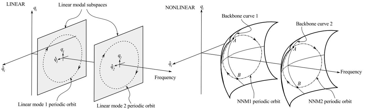
Fig. 5. Schematic drawing of two linear and nonlinear modal subspaces and manifold nonlinear normal mode (NNM) concept.
