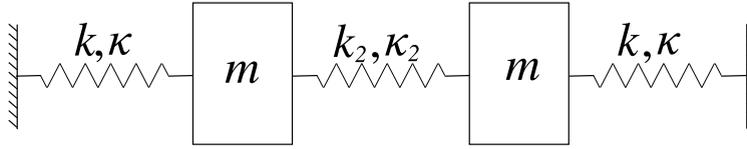
Fig. 2. The two degree-of-freedom example.
