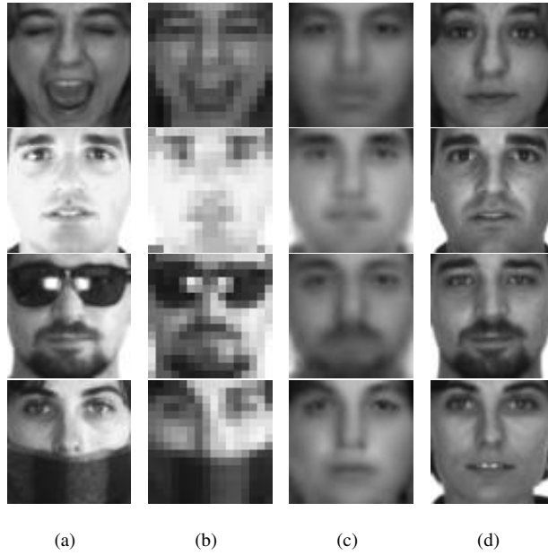
Figure 6: Representative results with upscaling \times 4 . (a) Raw test images with intra-personal variations. (b) Input LR images. (c) Images recovered by proposed method. (d) Ground truth.
