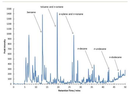
Fig. 2 1D GC chromatogram from a winter ClearfLo GCxGC chromatogram (using Zoex GC Image software) with three major aromatics and the C8–C12 n-alkanes identified. Reproduced with permission from Dunmore  $et al.^{1}$
