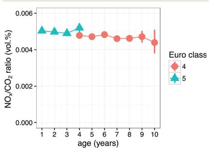
Fig. 4  $NO_x/CO_2$  ratio for Euro 4 and Euro 5 diesel passenger cars as a function of vehicle age
