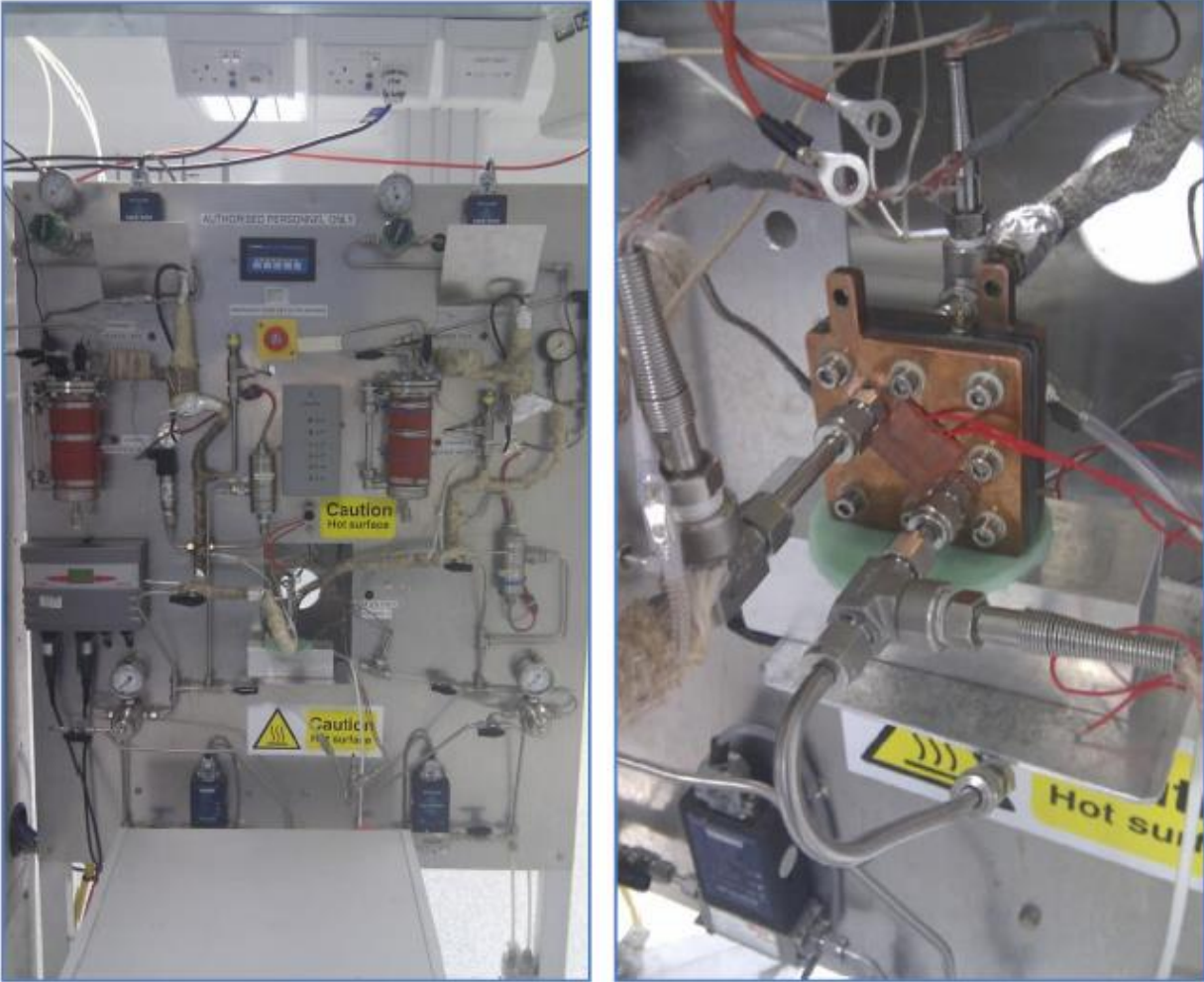
Figure 5: (A) PEM fuel cell test-rig at University of Leeds. (B) Close-up of complete MEA fuel cell assembly with the anodic surface in the foreground connected to dihydrogen inlet and outlet supply. The cathodic reverse side is supplied with air, within which dioxygen acts as ultimate electron acceptor.
