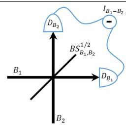
**Figure 2.** Diagram to represent the two channel system undergoing balanced homodyne detection, where  $B_1$  is the input signal (mode D in protocol), and  $B_2$  is the local oscillator.  $I_{B_1-B_2}$  is the intensity difference between the photodetectors  $D_{B_1}$  and  $D_{B_2}$ .
