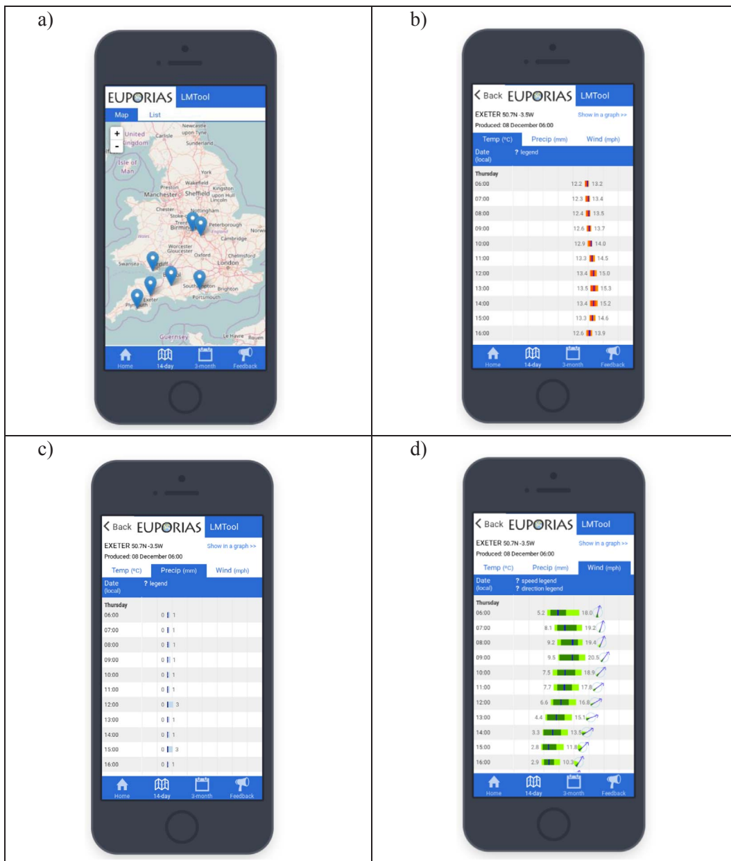
Fig. 7. The mobile app developed for the LMTool prototype, showing a) the location map, and examples of 14-day forecasts for Exeter for b) temperature, c) precipitation and d) wind speed/direction. The app is freely available for both Android and Apple iOS, while the data is not freely available and requires a pass-code. Legends for b-d are as in Fig. 6.
