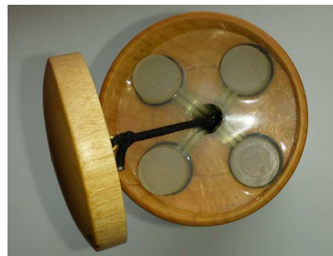
Fig. 5: Top view with removed excitation pad, showing the four silicone cushions with FSRs below
