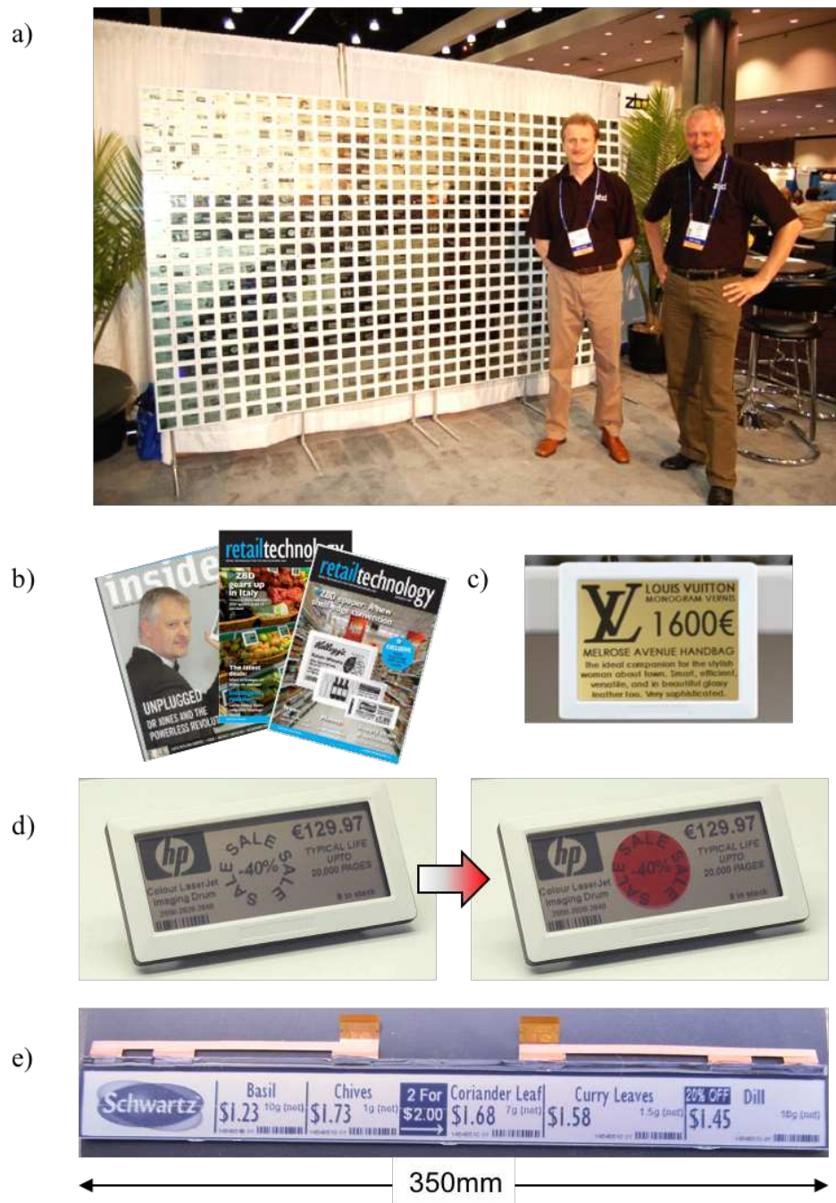
Figure 10 Marketing the ZBD technology. a) ZBD at SID 2008. The 43-million pixel display: 560 QVGA epop labels addressed using the ZBD proprietary Bounce RF communications system. b) Most publications were in trade magazines, rather than technical journals. Items from the Malvern concept centre included c) displays with different colour options, d) an operational colour shutter that allowed three colours to be displayed on an epop label, and e) a 14" wide shelf-strip demonstrator.
