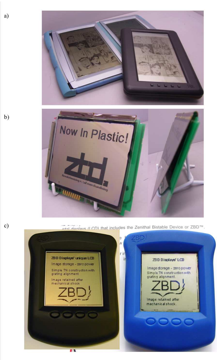
Figure 4 Progress made during the first two-years. a) Two page ZBD E-book Reader (Z-book) concept and the 7" demonstrator. These were among the first demonstrators to include the TN ZBD variant. b) Plastic VGA display [21]. c) Improvements to the optics and manufacturing dominated the R&D in this period, represented by move from the black to blue demonstrators as shown. The use of embossing for the demonstrator on the right allowed a transparent photopolymer and the improved, near sinusoidal grating shape with low pre-tilt and consequently wider viewing angle. These early prototypes used a display that mimicked that used in the Palm V PDA.
