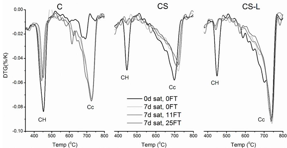
**Figure 4.** Portlandite and calcium carbonate contents during cyclic freezing and thawing of the investigated cements
