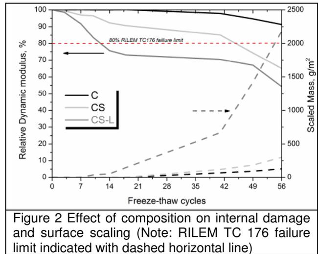
Figure 2 Effect of composition on internal damage and surface scaling (Note: RILEM TC 176 failure limit indicated with dashed horizontal line)
