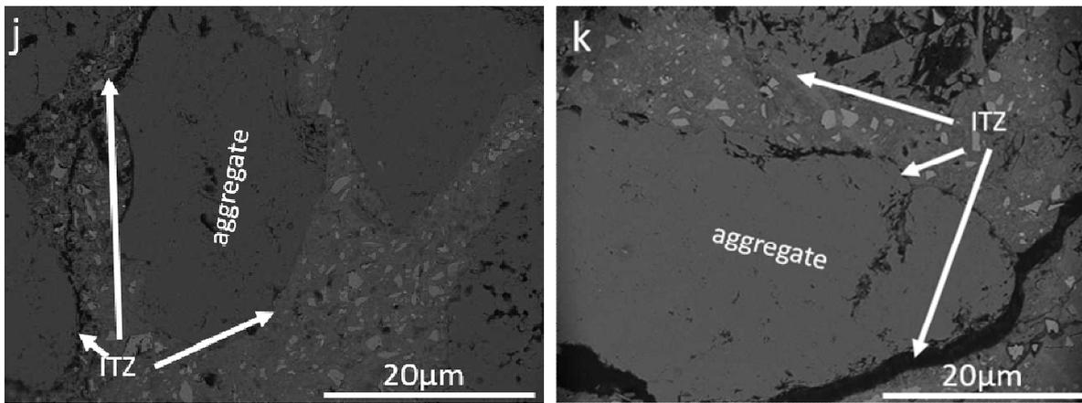
**Figure 3.** Microstructural changes associated with freeze-thaw of composite cements (Images obtained from 5mm concrete slices partially immersed in DIW for 25 freeze-thaw cycles)
