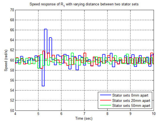
Fig. 7: Speed responses of the rotor, R_1 with 0mm ( D_S = 65mm , according to Fig 3), 20mm ( D_S = 85mm ) and 50mm ( D_S = 115mm ) distance between stator set 1 and stator set 2 (inter-set distances), focusing only on the response when stator set 2 is switched on at 5 seconds.
