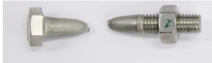
Stainless steel - failure by ductile body necking
