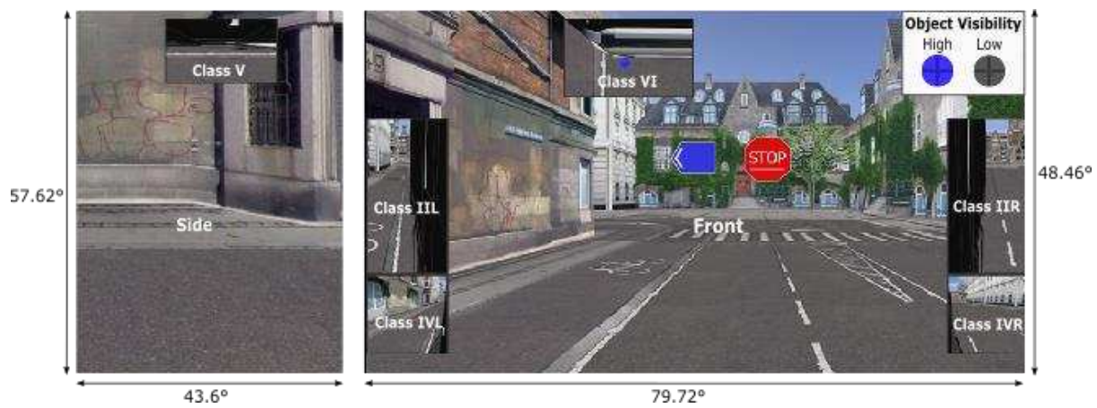
Figure 2. Simulator screenshots annotated with labels for windows and mirrors and high-visibility (Blue) and low-visibility (Grey) objects enlarged and super-imposed onto the screenshot (top-right hand corner). The high-visibility object is visible in the driver's Class VI mirror. The screenshot shows a driver approaching a zebra crossing. The 'Stop' sign instructs the driver to come to a complete stop until the 'Stop' sign flips to 'Go', whereupon they can turn move off and turn left.
