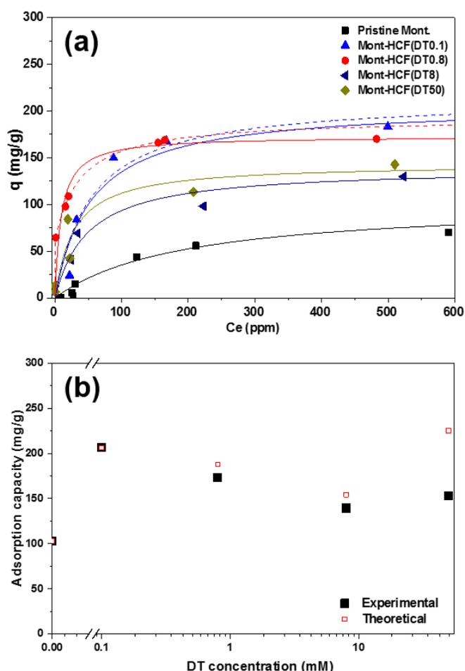
**Figure 6.** a) Cs<sup>+</sup> adsorption isotherm as a function of the equilibrium concentration ( $C_e$ ) for Mont-HCF composites and pristine montmorillonite. Solid and dashed lines represent fittings by the Langmuir model (solid) and Dual-site Langmuir model (dashed). b) Comparison between the experimental and theoretical maximum adsorption capacities,  $q_m$ , for Mont-HCF composite particles as a function of DT concentration.
