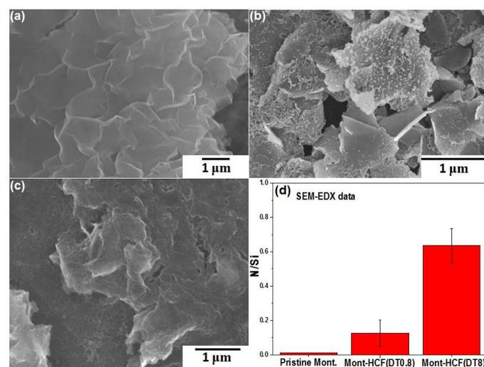
**Figure 4.** SEM images of a) pristine montmorillonite, b) Mont-HCF(DT0.8), c) Mont-HCF(DT8) composites, and d) N/Si ratio determined from SEM-EDX analysis.
