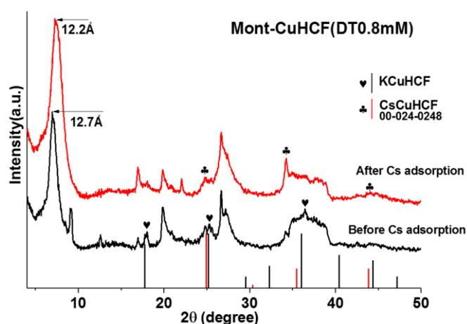
**Figure 7.** XRD patterns of Mont-HCF(DT0.8) before and after Cs<sup>+</sup> adsorption (pattern file 00-024-0248 for CsCuHCF).
