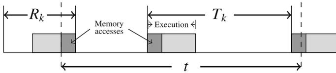
**Fig. 2** Illustration of the carry-in interference analysis
