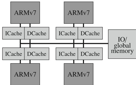
frequency of 200 MHz. Each core has separate instruction and data caches, both direct-mapped with 512 cache sets each and a block size of 32 Bytes. The global memory latency  $d_{\text{main}}$  and the DRAM refresh latency  $d_{\text{refresh}}$  are both 5 cycles. The DRAM refresh period  $T_{\text{refresh}}$  is 64 ms. We assume the DRAM implements the distributed refresh strategy (see Sect. 6.4).
