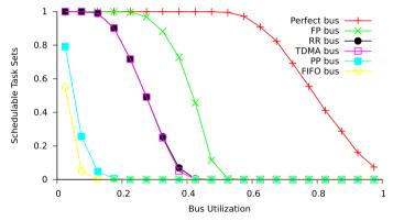
Fig. 6 Number of schedulable task sets versus bus utilization: varying bus arbitration policy
