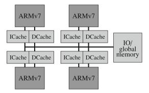
frequency of 200 MHz. Each core has separate instruction and data caches, both direct-mapped with 512 cache sets each and a block size of 32 Bytes. The global memory latency  $d_{\text{main}}$  and the DRAM refresh latency  $d_{\text{refresh}}$  are both 5 cycles. The DRAM refresh period  $T_{\text{refresh}}$  is 64 ms. We assume the DRAM implements the distributed refresh strategy (see Sect. 6.4).
