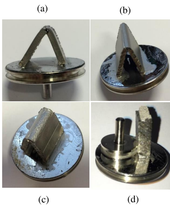
Fig.2: Samples prepared for SEM by mechanical fracturing for anodised alloys (a) M, (b) H, (c) F and (d) A.
