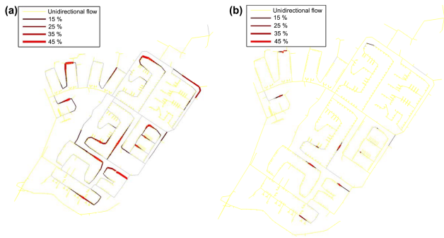
Figure 4. The fraction of time that the flow reverses in a model with (a) bottom-up allocated SIMDEUM demands (Blokker, 2010) and (b) top-down demand allocations. The 50 % value means that 50 % of the time the flow is in one direction and 50 % in the other.
