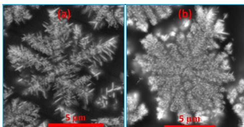
**Figure 14.** Backscattered SEM images of samples with (a) one crystallization stage (nucleation at 810 °C for 2 h, crystal growth at 1000 °C for 2 h) and (b) two crystallization stages (nucleation at 810 °C for 2 h and crystal growth at 900 °C for 10 h and then at 1000 °C for 2 h).
