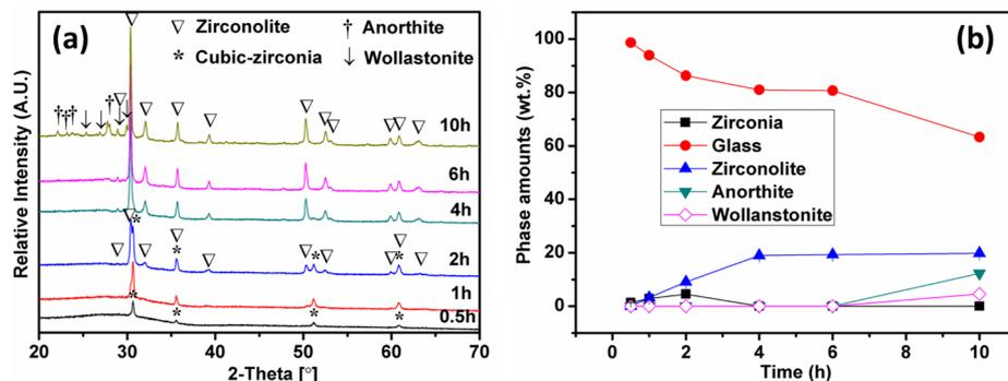
**Figure 5.** XRD phase-identification results (a) and quantification results (b) of samples prepared by nucleation at 810 °C for 2 h followed by crystal growth at 950 °C for different dwelling times ( $t = 0.5, 1, 2, 4, 6,$  and  $10$  h).
