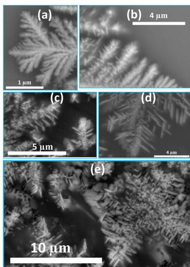
Figure 10. Backscattered SEM images of samples prepared by nucleation at 810 °C for 2 h followed by crystal growth at 1000 °C for different dwelling times *t*, (a) *t* = 10 min; (b) *t* = 0.5 h; (c) *t* = 2 h; (d) *t* = 4 h; (e) *t* = 10 h, showing the details of crystal evolution from cubic-zirconia to zirconolite and the crystal growth of zirconolite.
