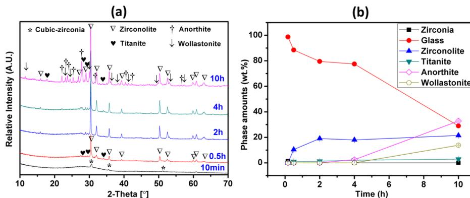
**Figure 8.** XRD phase-identification results (a) and quantification results (b) of samples prepared by nucleation at 810 °C for 2 h followed by crystal growth at 1000 °C for different dwelling times ( $t = 10$  min, 0.5, 2, 4, and 10 h).
