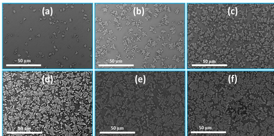
**Figure 6.** Backscattered SEM images of samples prepared by nucleation at 810 °C for 2 h followed by crystal growth at 950 °C for different dwelling times  $t$ , (a)  $t = 0.5$  h; (b)  $t = 1$  h; (c)  $t = 2$  h; (d)  $t = 4$  h; (e)  $t = 6$  h; (f)  $t = 10$  h.
