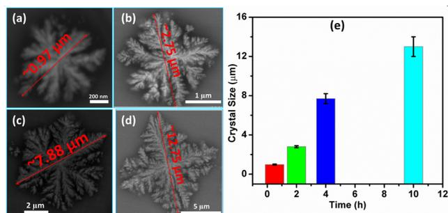
**Figure 3.** Backscattered SEM images of representative crystal in samples prepared by nucleation at 810 °C for 2 h followed by crystal growth at 900 °C for different dwelling times  $t$ , (a)  $t = 0.5$  h; (b)  $t = 2$  h; (c)  $t = 4$  h; (d)  $t = 10$  h; (e) crystal size of samples prepared by nucleation at 810 °C for 2 h followed by crystal growth at 900 °C for different dwelling times ( $t = 0.5, 2, 4,$  and  $10$  h).
