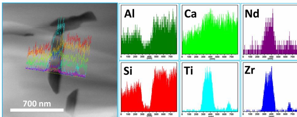
Figure 9. TEM-EDX line-scan profiles of the elements Al, Ca, Nd, Si, Ti, and Zr across the zirconolite crystal.
