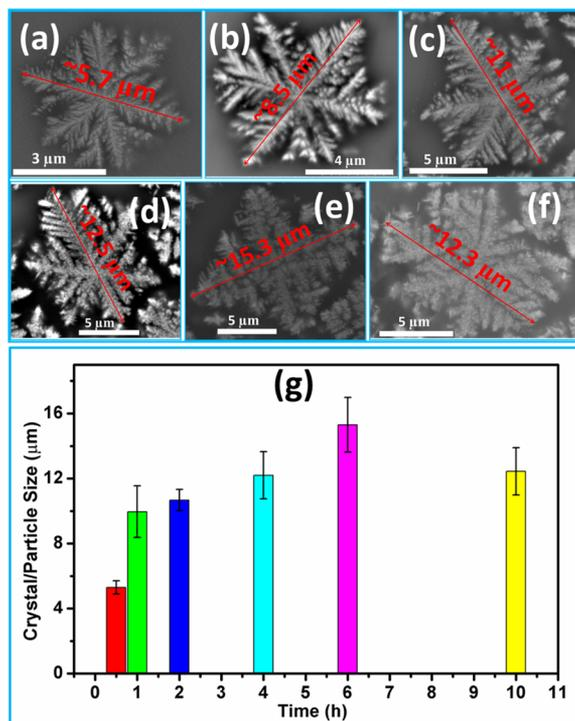
**Figure 7.** Backscattered SEM images of representative crystals in samples prepared by nucleation at 810 °C for 2 h followed by crystal growth at 950 °C for different dwelling times  $t$ , (a)  $t = 0.5$  h; (b)  $t = 1$  h; (c)  $t = 2$  h; (d)  $t = 4$  h; (e)  $t = 6$  h; (f)  $t = 10$  h; (g) crystal size of samples prepared by nucleation at 810 °C for 2 h followed by crystal growth at 950 °C for different dwelling times ( $t = 0.5, 1, 2, 4, 6,$  and  $10$  h).
