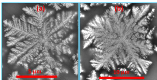
**Figure 13.** Backscattered SEM images of samples with (a) one crystallization stage (nucleation at 810 °C for 2 h, crystal growth at 950 °C for 2 h) and (b) two crystallization stages (nucleation at 810 °C for 2 h and crystal growth at 900 °C for 10 h and then at 950 °C for 2 h).
