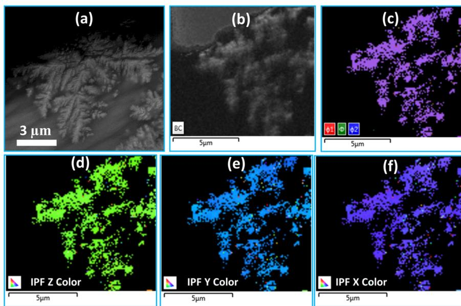
**Figure 4.** Electron backscatter diffraction results for sample prepared by nucleation at 810 °C for 2 h followed by crystal growth at 900 °C for 10 h, (a) Backscattered SEM image for the measured crystal; (b) band contrast for the measured area; (c) Euler angle map; (d) inverse pole figure (IPF) along the  $z$ -axis; (e) IPF along the  $y$ -axis; (f) IPF along the  $x$ -axis. In the IPF map, each color represents one orientation.
