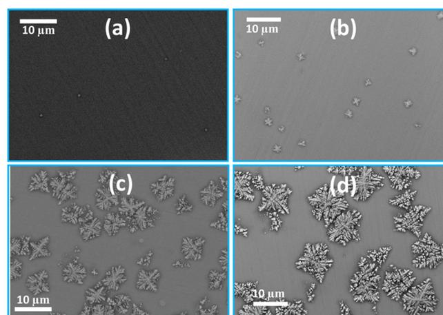
**Figure 2.** Backscattered SEM images of samples prepared by nucleation at  $810^\circ\text{C}$  for 2 h followed by crystal growth at  $900^\circ\text{C}$  for different dwelling times  $t$ , (a)  $t = 0.5$  h; (b)  $t = 2$  h; (c)  $t = 4$  h; (d)  $t = 10$  h.
