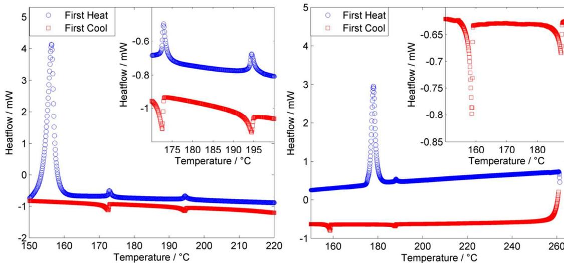
**Figure 4:** DSC thermograms for **O4**<sub>7</sub> with an expansion of the region between 170-200 °C (left) and for **O6**<sub>7</sub> with an expansion of the region between 150-190 °C (right). Both thermograms were obtained using a heat/cool rate of 10 °C min<sup>-1</sup>.
