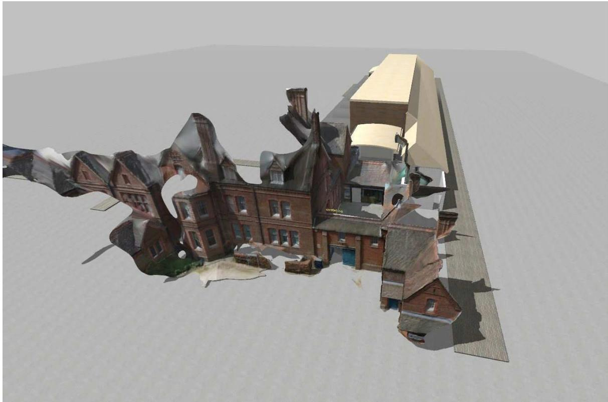
Figure 9: Combined model, incorporating the MERL entrance façade, the inner courtyard (both photogrammetry), and the main galleries (SketchUp)
