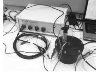
Fig. 3 Test setup for corrosion monitoring
