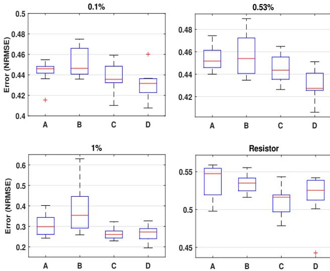
Fig. 3: Analysis of new features when added to each material: *test set* error decreases when input-weighting is used, and in some cases decreases further when time-scaling also used. Four combinations are assessed over 10 evolutionary runs: (A) No features used, i.e. applying only control signals with no time-scaling; (B) control signals and *time-scaling*; (C) *input-weighting* with no time-scaling; (D) both *input-weighting* and *time-scaling* applied to the reservoir.
