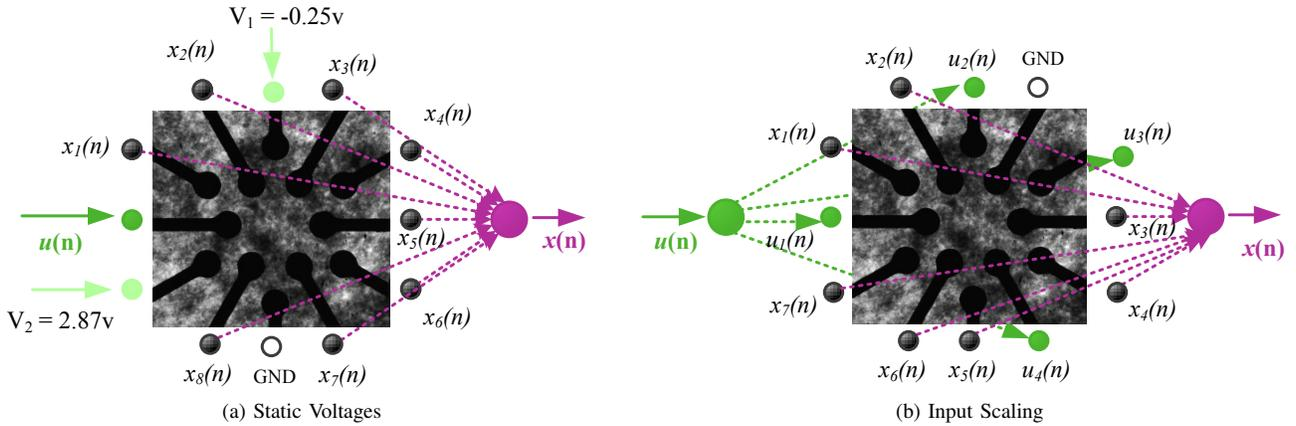
Fig. 1: Examples of the two input mechanisms used; a) configuration through static voltages (based on evolution *in materio* technique), and b) using multiple weighted inputs to various locations on the array (based on reservoir model). In the input-weighting scheme each input  $u_i(n)$  is multiplied by a weight stored in the genotype.
