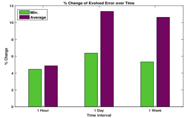
Fig. 5: A graph of the percentage change in error from the original evolved *test set* NRMSE of 0.195 over different time periods. This is shown for the best reservoir found with the SWCNT/PBMA 1% material using both time-scaling and input-weighting.
