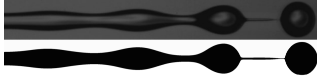
FIG. 6. A comparison of a video snapshot from the ROJER experiment (above) and the CFD result (below) using a 74% glycerol solution ( We = 17.4, Oh = 0.293 ).
