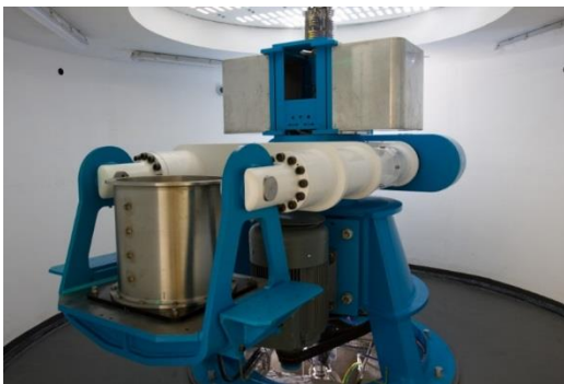
Figure 1. UoS-50gT 4m diameter centrifuge.
