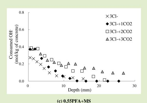
Fig. 6. Consumed OH<sup>-</sup> in concretes exposed to the 3Cl<sup>-</sup>+yCO<sub>2</sub> regime
