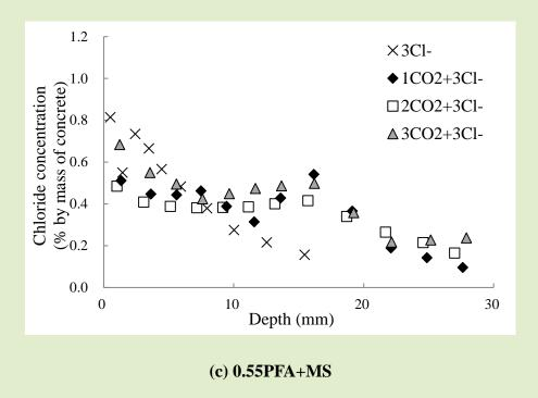
Fig. 11. Distribution of Cl<sup>-</sup> in concretes exposed to yCO<sub>2</sub>+3Cl<sup>-</sup> regime
