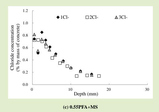
Fig. 3. Distribution of Cl- in concretes during the xCl- regime
