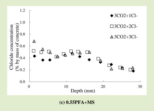
**Fig. 10.** Distribution of Cl<sup>-</sup> for the 3CO<sub>2</sub>+xCl<sup>-</sup> regime
