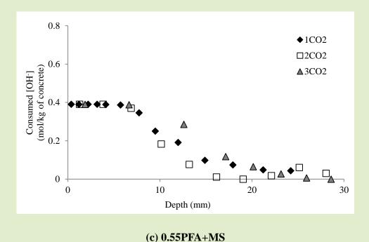
Fig. 9. Consumed OH<sup>-</sup> during the three months of carbonation
