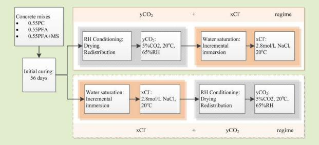
Fig. 2. Flowchart of the experimental processes
