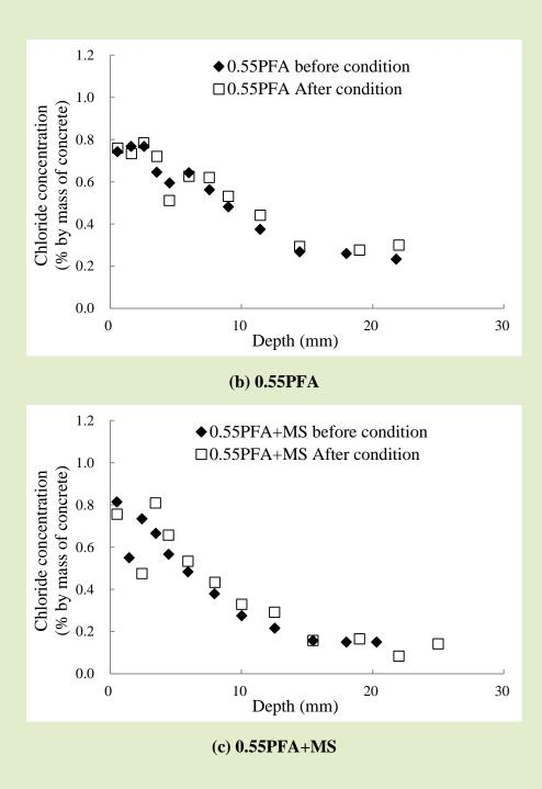
Fig. 4. Distribution of Cl<sup>-</sup> before and after the condition of RH
