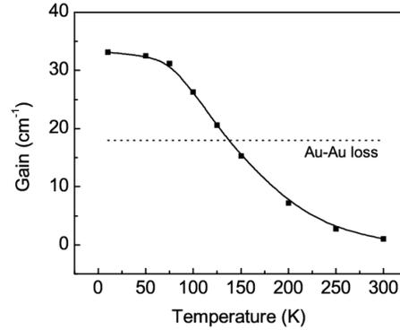
Fig. 2. Calculated unclamped peak gain of the design as a function of the lattice temperature. The dotted line shows the calculated optical loss in a QCL with a gold–gold waveguide configuration.
