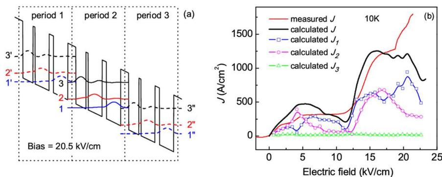
Fig. 1. (a) Calculated conduction band diagram and squared moduli of bound electronic wave functions of a three-well design at an electric field of 20.5 kV/cm. (b) Comparison between the calculated and measured I–V curves, and the calculated resonant tunnelling current from each subband to the downstream period versus electric field.  $J_1$ ,  $J_2$  and  $J_3$  indicate the current density extracted from the subband levels 1, 2 and 3, respectively.
