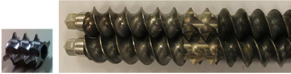
Figure 1 – Picture of (left) distributive feed screw (DFS) and (right) screw configuration with conveying elements (CEs) used. The pitch length of the conveying elements (CEs) and the DFS element is 0.5D . Figure 1
