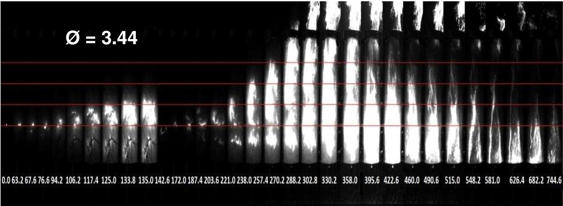
**Oak sieved to give the size range 63 - 150 $\mu\text{m}$  ( $\text{Ø}=1= 218.9$ ) 1 g, 750g/m<sup>3</sup>,  $\text{Ø}=3.44$**
