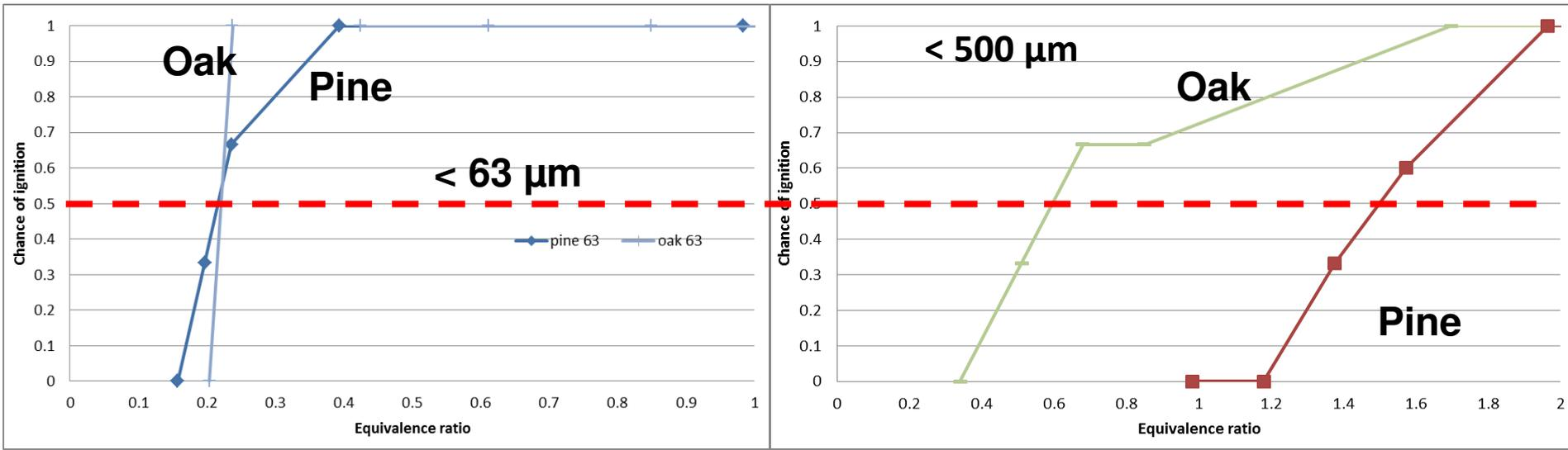
**The differences in MEC between oak and pine dusts was due to differences in the actual particle size distribution for the same sieve size. It was not due to any chemical differences in the particles.**
