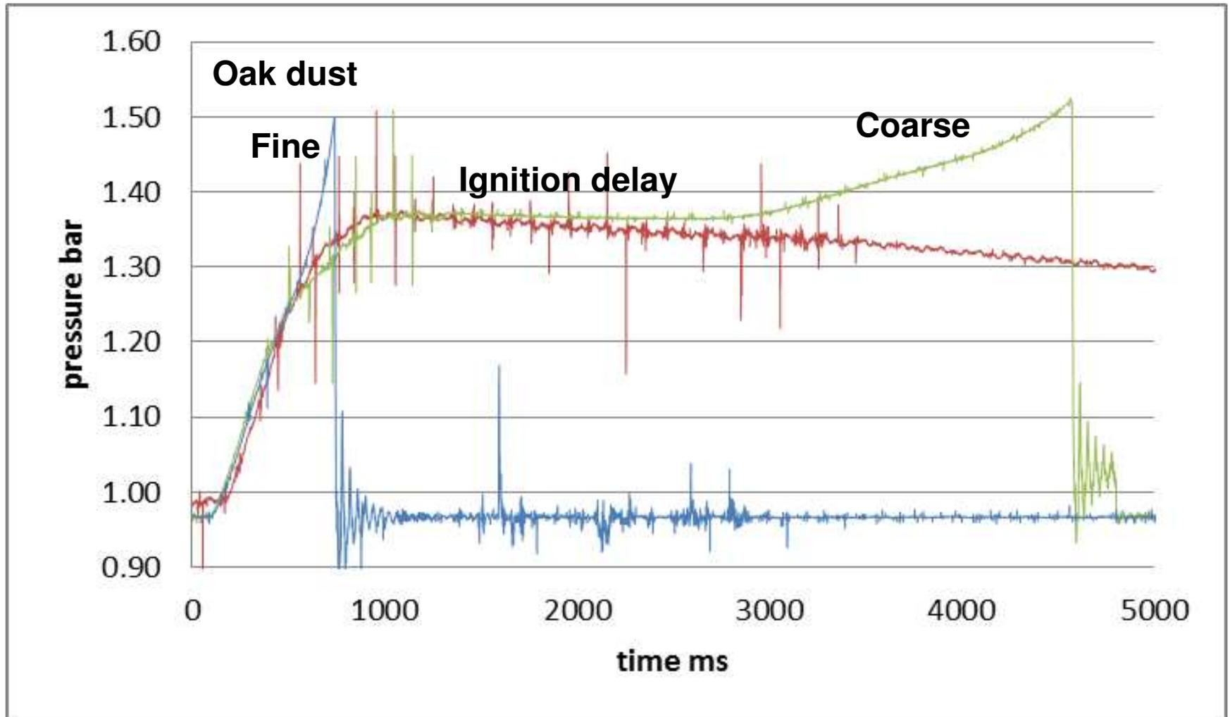
Without dust (red), With dust - coarse and ignition (green) and With dust - fine and ignition (blue)
