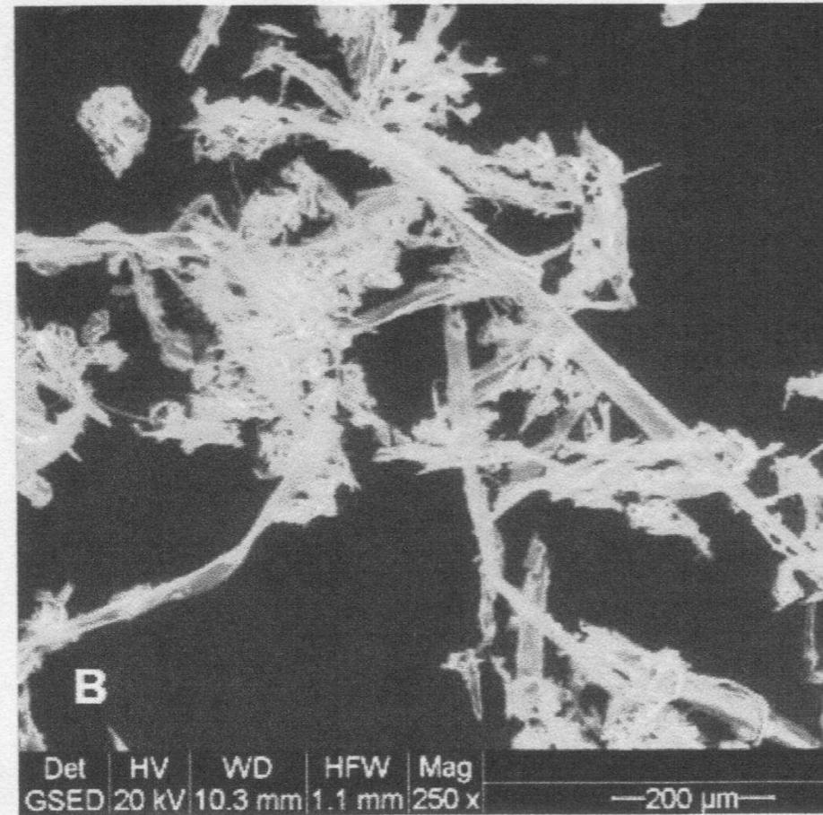
**SEM analysis of wood sawdust that passed through a 1mm sieve but were Retained by a 425 μm sieve.**
