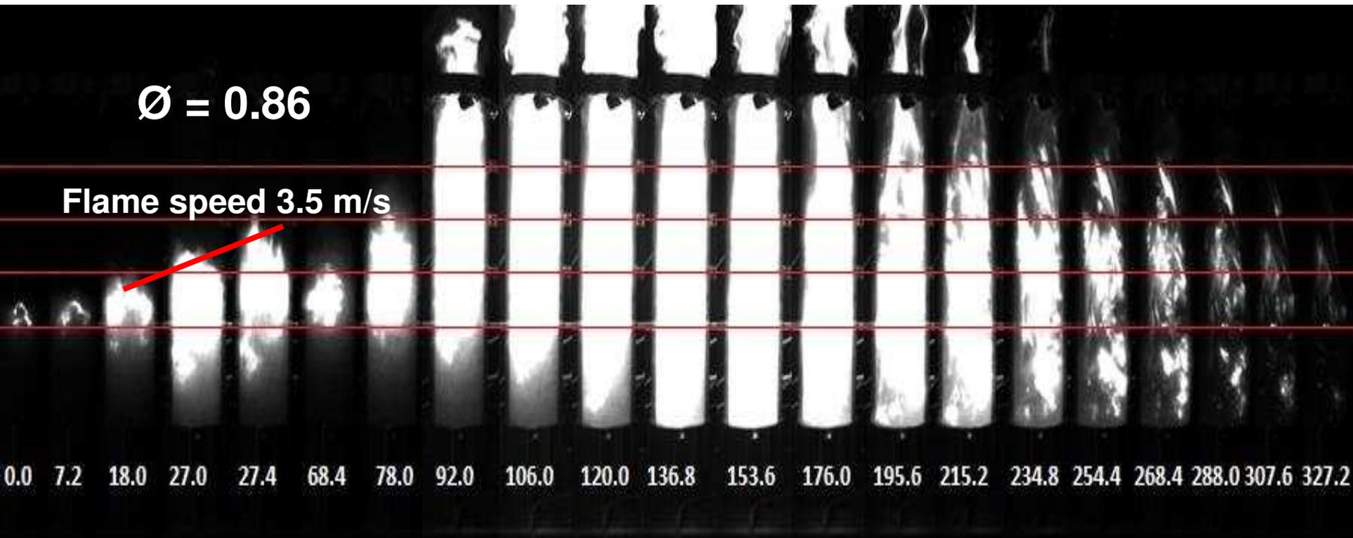
**Oak sieved to  $< 63\mu\text{m}$  ( $\text{Ø}=1= 218.9$ ) 0.25 g,  $187.5\text{g}/\text{m}^3$ ,  $\text{Ø}=.86$**
