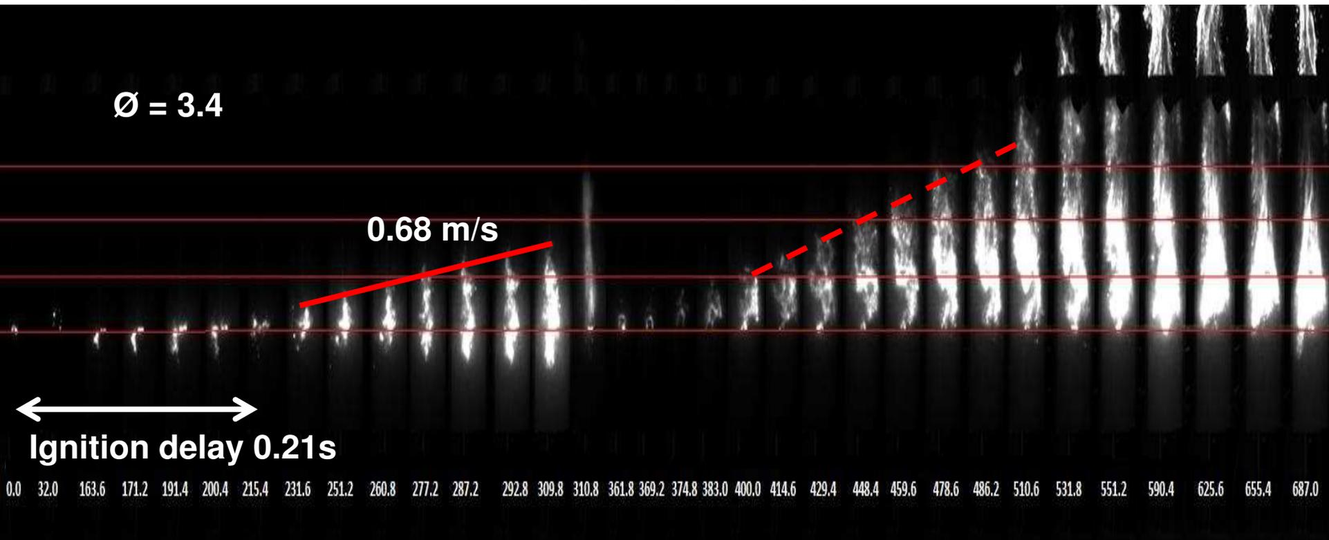
**Oak dust sieved to  $<500\mu\text{m}$  ( $\text{Ø}=1= 218.9$ ) 1 g,  $750\text{g}/\text{m}^3$ ,  $\text{Ø}=3.44$**
