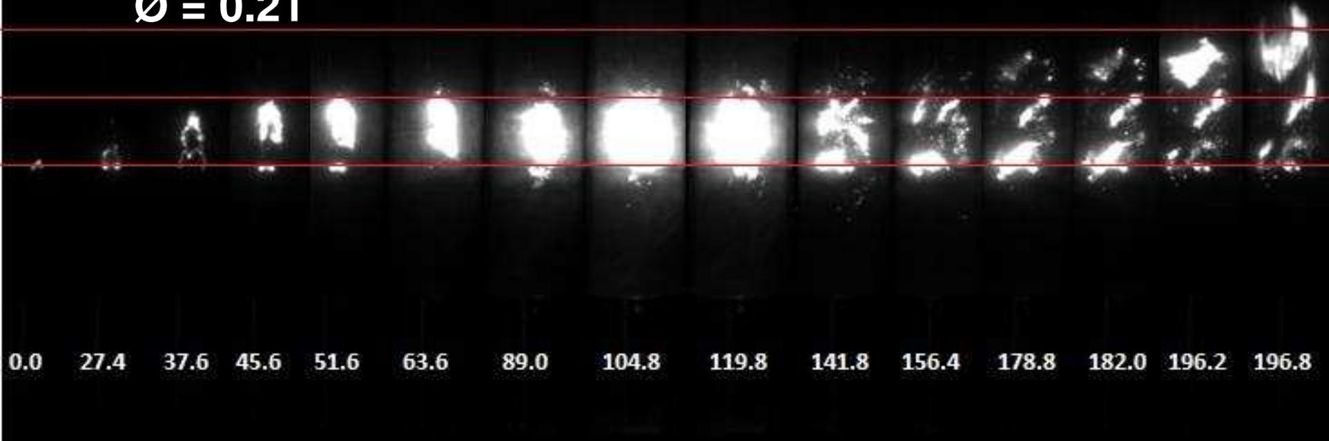
**Oak 63 – 150  $\mu\text{m}$  ( $\varnothing=1= 218.9$ ) 0.06 g, 45g/m<sup>3</sup>,  $\varnothing=0.206$**
