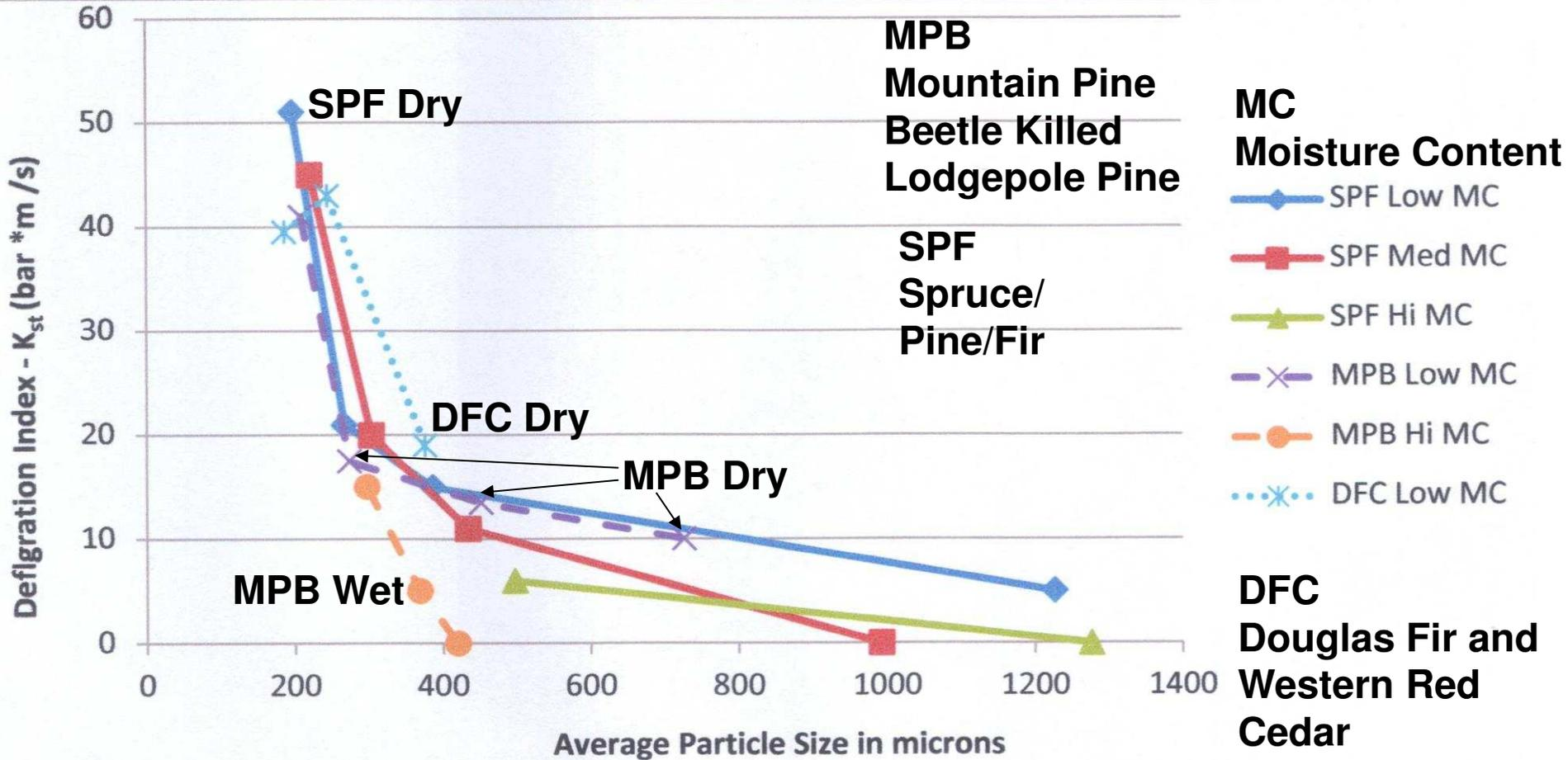
$K_{st} = dp/dt_{max} V^{0.33}$  bar m/s which is a measure of the dust reactivity
