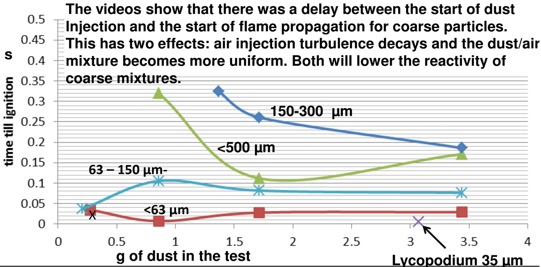
The time from the start of injection to the video observation of the start of flame propagation for oak sawdust. The size fractions were achieved by sieving. Fine particles have the lowest delay and the presence of fines with coarse particles reduces the overall ignition delay.
