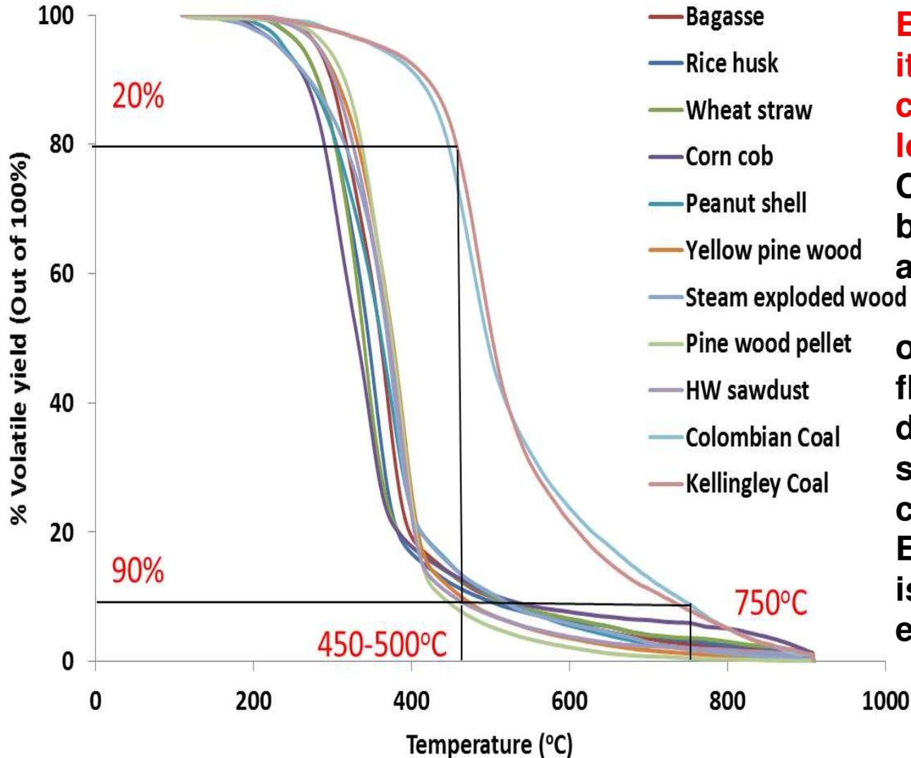
**Biomass has lost 90% of its volatiles by 400°C compared with only 10% loss of volatiles for coal. Combustion air in coal burners is preheated to around 300°C where there is typically 30% volatile of volatiles in biomass flames will make a large difference in the flame structure compared with coal flames. Early release of volatiles is also crucial in the explosion hazards and in the biomass reactivity.**
