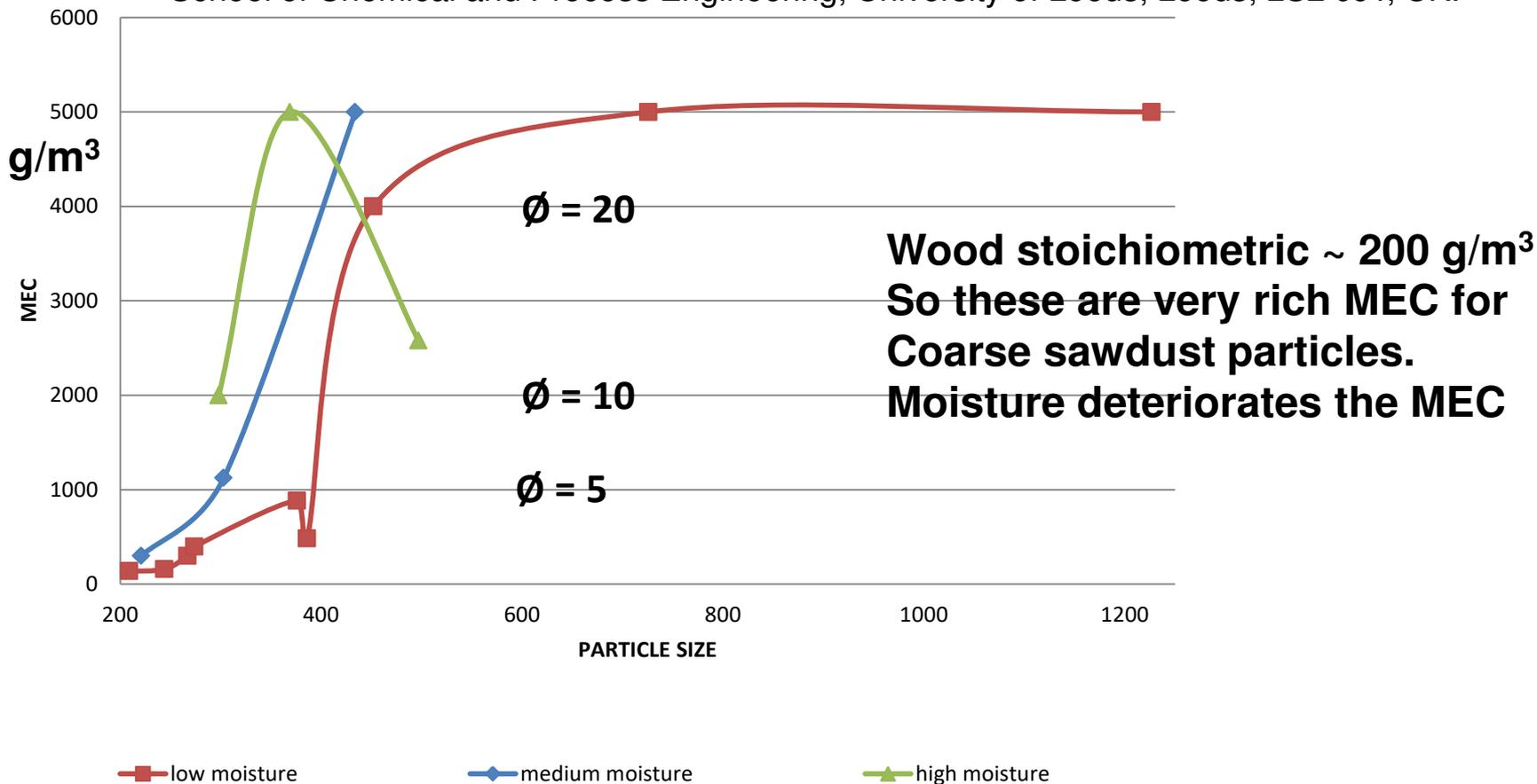
**MEC data for sawdust for large particles. MEC as high as 5000 g/m<sup>3</sup>.
