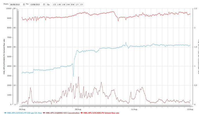
Fig. 6. PDO Harweel GSU Gas outlet responses with a set point increment of 33% in gas flow rate. Blue: Gas flow rate (Range 0 - 2.5 MMSCMD), Brown: H 2 S concentration (Range 0 - 50 ppm), Red: Solvent flow rate (Range 0 - 10000 m 3 /d)
