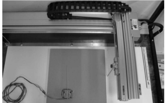
Fig. 1. The XY positioning robot. The whisker was deflected by the robot along the X axis through movements in a clockwise or anticlockwise direction as viewed from above.
